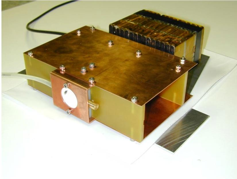
Figure 1 PPT-7 Coaxial electrothermal pulsed plasma thruster
