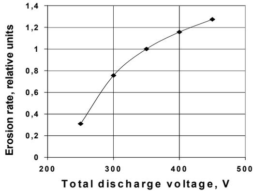
**Figure 1. Dependence of the insulator erosion rate from the discharge voltage under the constant mass flow rate through the source anode  $\dot{m}_{anode} = 2.0 \text{ mg/s}$  and the cathode  $\dot{m}_{cathode} = 0.4 \text{ mg/s}$ .**
