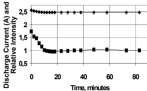
**Figure 2. Discharge current (rhombus) and line BI relative intensity (squares) as a function of time under  $\dot{m}_{anode} = 2.5 \text{ mg/s}$ ;  $\dot{m}_{cathode} = 0.4 \text{ mg/s}$ ;  $U_d=350 \text{ V}$ .**
