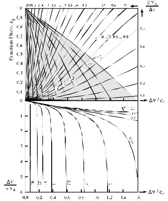
Fig. 4: Nomograph of the quantities  $\Delta v$ ,  $t_I^*$ ,  $m_{LS}$ , and  $c_e$  for the optimized rocket equation for high power thermal arcjets, ion, Hall ion and MPD thrusters
