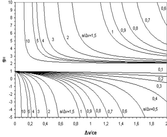
Fig. 7: Function of  $g_{II}$  vs.  $\Delta v/c_e$  with the mission and propulsion system dependent parameter  $a/\Delta v$
