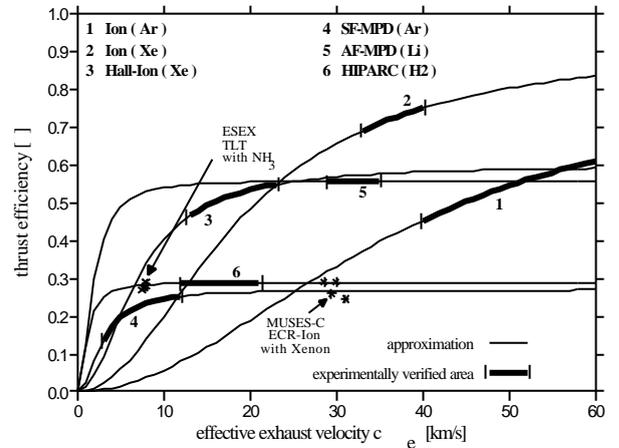
**Fig. 3: Thruster efficiency vs. effective exhaust velocity for different thrusters (see Table 2)**
