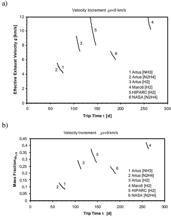
Fig. 14: Effective exhaust velocity  $c_e$  (a), payload and structure mass fraction  $\mu_{LS}$  (b) vs. flight time  $\tau$  for thermal arcjet thrusters (Table 3) for a velocity increment of  $\Delta v = 9$  km/s
