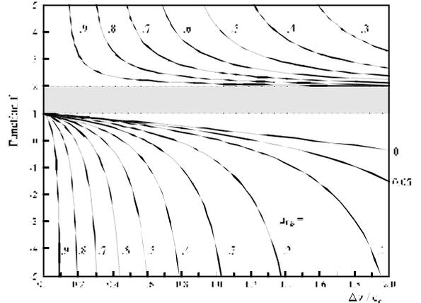
Fig. 1: Function  $f$  vs  $\Delta v/c_e$  with the payload plus structure mass fraction  $\mu_{LS}$  as parameter
