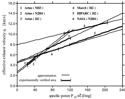
Fig. 5: Effective exhaust velocity  $c_e$  as function of specific power for different thermal arcjet thrusters and propellants (see Table 3)
