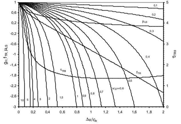
Fig. 10: Diagram of  $\Delta v, c_e, \mu_{LS}$  and  $\tau_{TR,II}^*$  for thermal arcjet thrusters for the case of an optimized transport rate
