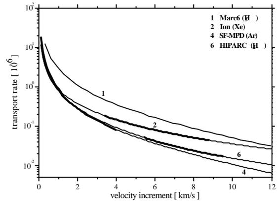
Fig. 17: Transport rate as a function of velocity increment [km/s] for selected thrusters
