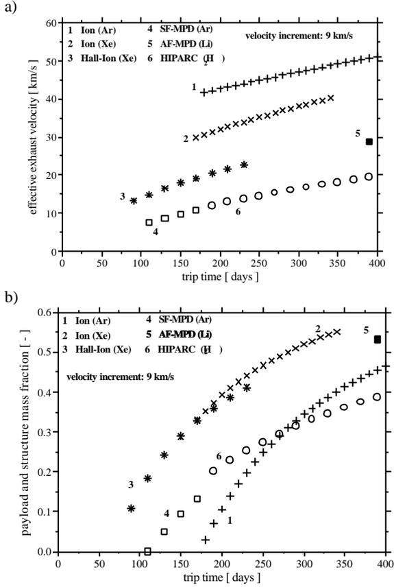
Fig. 12: Effective exhaust velocity  $c_e$  (a), payload and structure mass fraction  $\mu_{LS}$  (b) vs. flight time  $\tau$  for thrusters in Table 2 for a velocity increment of  $\Delta v=9\text{km/s}$
