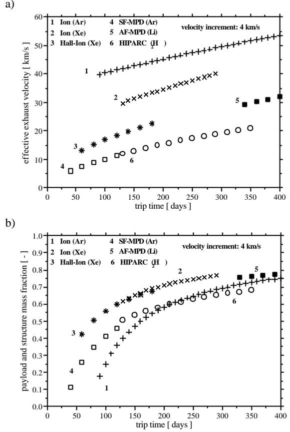
Fig. 11: Effective exhaust velocity  $c_e$  (a) , payload and structure mass fraction  $\mu_{LS}$  (b) vs. flight time  $\tau$  for thrusters in Table 2 for a velocity increment of  $\Delta v = 4\text{km/s}$
