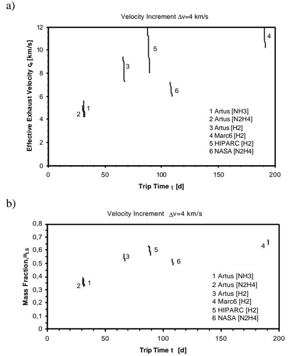
Fig. 13: Effective exhaust velocity  $c_e$  (a), payload and structure mass fraction  $\mu_{LS}$  (b) vs. flight time  $\tau$  for thermal arcjet thrusters in Table 3 for a velocity increment of  $\Delta v=4\text{km/s}$
