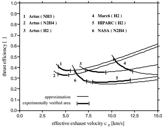
Fig. 6: Thrust efficiency  $\eta_T$  as function of effective exhaust velocity for different thermal arcjet thrusters and propellants (see Table 3)
