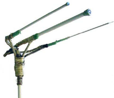
Figure 5. Flat probe 5 mm, flat probe 5 mm with guard ring, cylindrical probe (from left to right).
