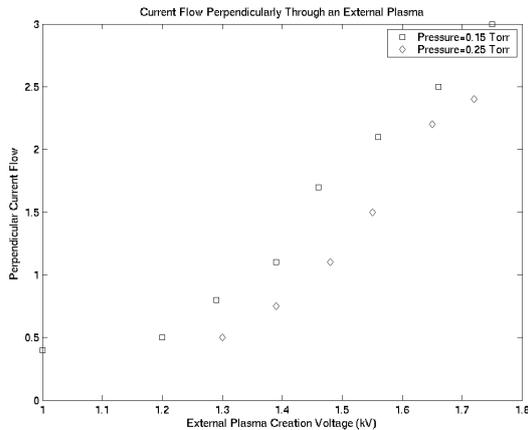
Figure 5: Current Flow between Two Probes Immersed in an External Plasma
