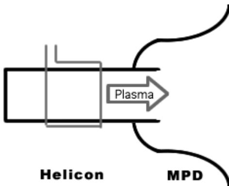
Figure 1: Design of a New Helicon MPD Thruster
