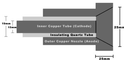
Figure 6: Cross Section of the Experimental "MPD" Thruster
