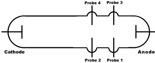
Figure 3: Glow Discharge Experimental Configuration
