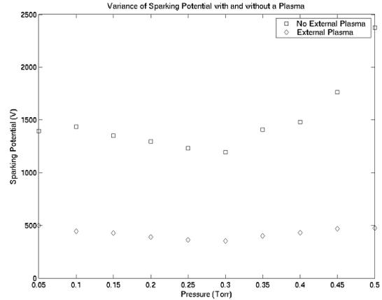
Figure 4: Sparking Potential with and without an External Plasma
