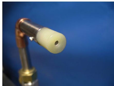
Figure 4. Photograph of miniaturized retarding potential analyzer (taken before the graphite shield is added). The total probe diameter is 15 mm. The front aperture is 4 mm in diameter.
