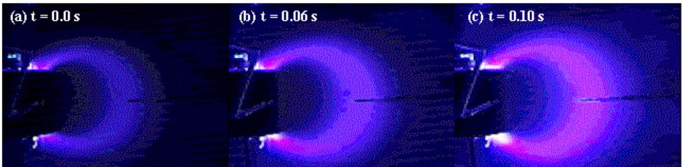
**Figure 3.** Optical emissions from a neutral puff during long duration testing. Time is from the introduction of the puff. The dark horizontal line of the right of each panel is a Langmuir probe. Field of view is  $\sim 40$  cm.
