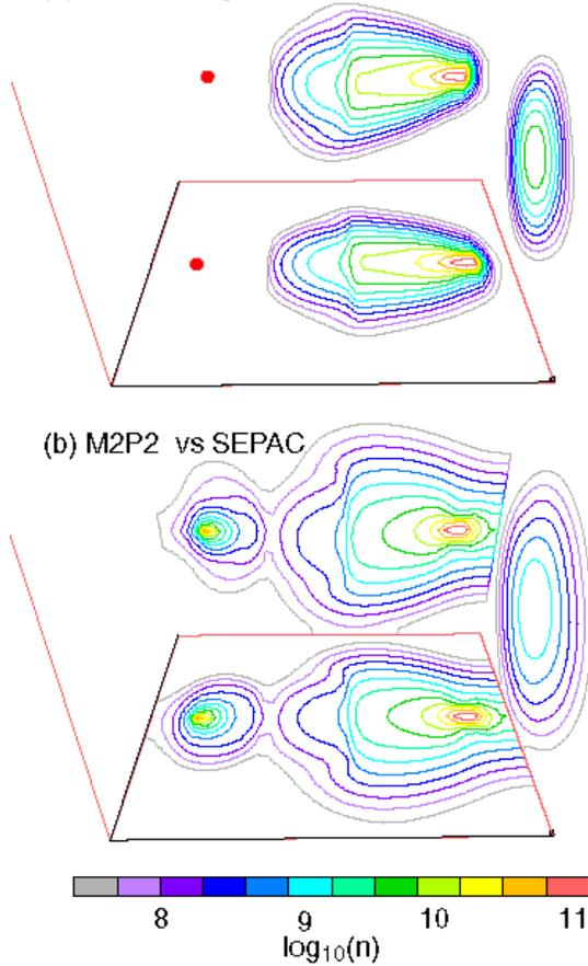
**Figure 5.** Density contours in  $\text{cm}^{-3}$  during (a) operation of the SEPAC source from 0-3.6 ms and (b) operation of the SEPAC source through  $t = 3.6$  ms with the M2P2 source on from 3.0 to 3.6 ms. The bottom contours of each panel show an equatorial cut through the center, the back contours a vertical cut through the center, and the right contours a cross-section through the model of the simulation box. The red dots in (a) show the position of the M2P2 source.
