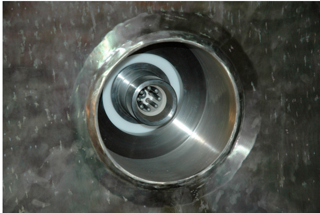
Figure 4. Discharge chamber on space chamber wall.
