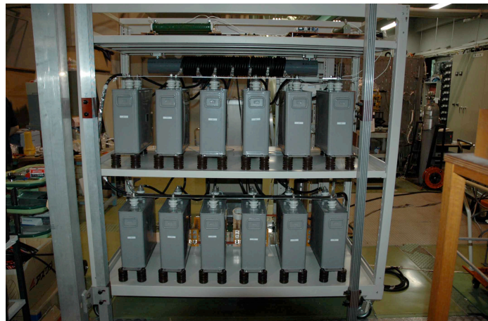
Figure 7. Photograph of the Pulse Forming Network (PFN).
