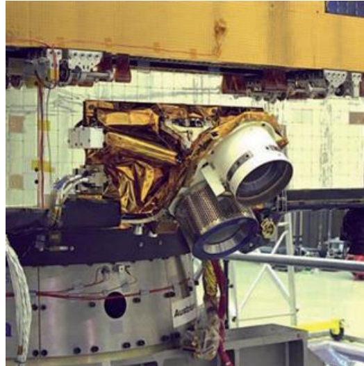
RIT-10 (white) and a British Kaufman- thruster UK-10 on ARTEMIS Courtesy of EADS
