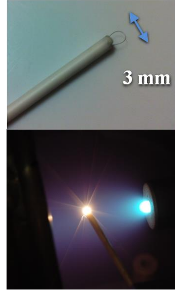
Figure 2. Emissive Probes. (Top) the alumina emissive probe body shown with tungsten filament. (Bottom) The emissive probe in floating point operation.
