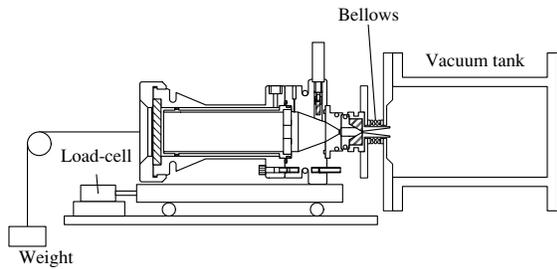
Figure 4: Thrust measurement system in vacuum.
