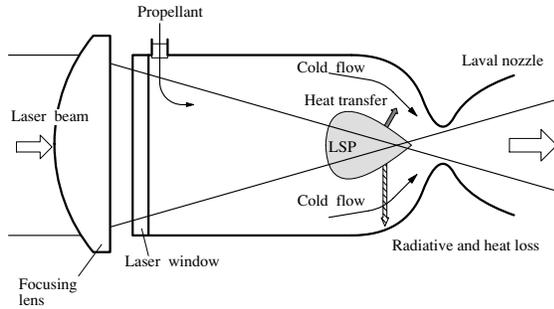
Figure 1: Concept of laser propulsion
