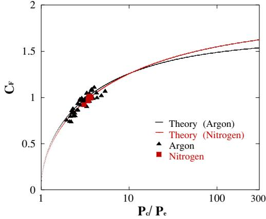
Figure 6: Thrust coefficient calculated using measured thrust and pressure as a function of pressure ratio.
