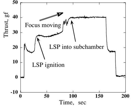
Figure 7: Time sequence of thrust at 700W and Ar 0.593 g/sec on thruster model II.
