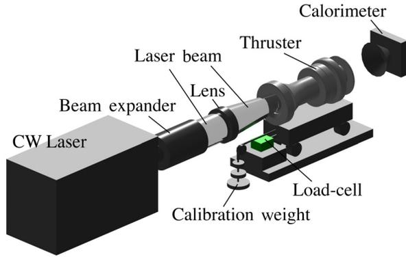
Figure 3: Schematic of thrust measurement system.
