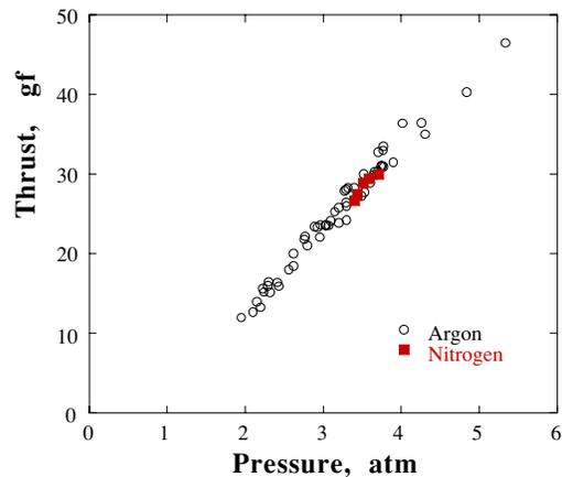
Figure 5: Relation between thrust and pressure on thruster model I.
