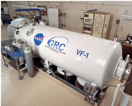
Figure 1. MPD thruster testing facility and pulsed power supply.
