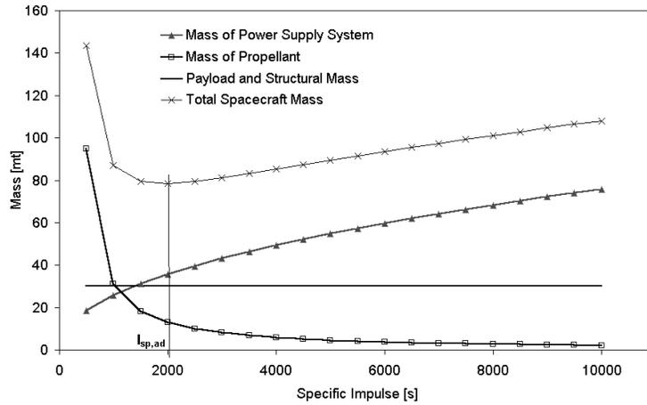
Figure 1. Mass versus specific impulse, qualitative diagram
