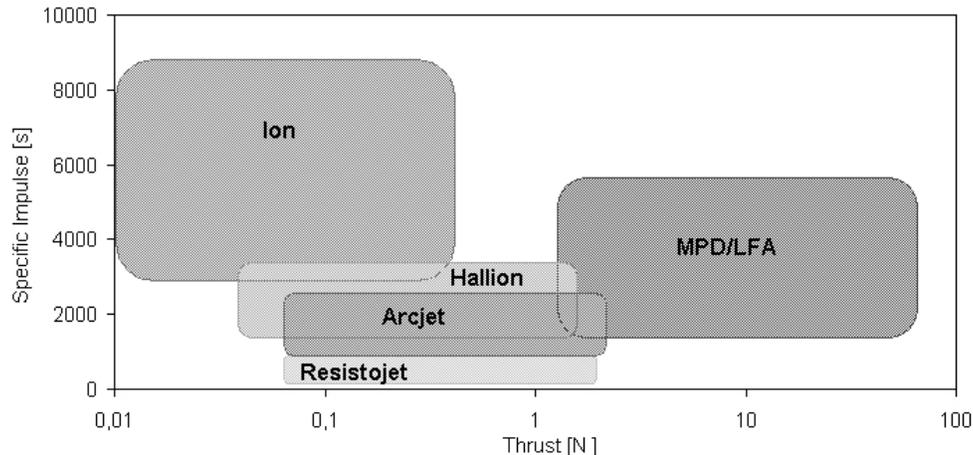
Figure 5. Thrust levels and specific impulses for different electric propulsion system concepts
