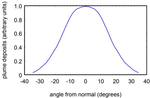
Figure 13. The angular distribution of the plume in a plane perpendicular to the tape direction.
