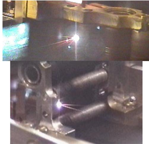
Figure 7. Two views of the thruster in operation.
