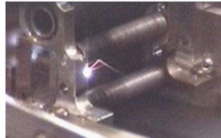
Figure 8. Ejected material reflecting off a guide roller.
