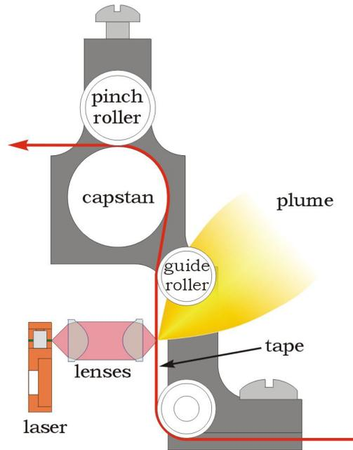
Figure 11. The location of the tape guide rollers, optical components, and exhaust plume.
