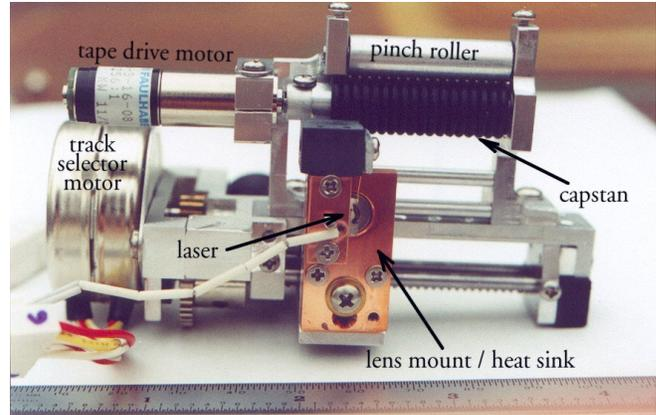
Figure 2. Selected parts of the preprototype thruster, looking in the direction of the laser propagation.
