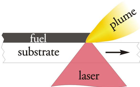
Figure 12. Plume steering by the edge of the ablated fuel material.
