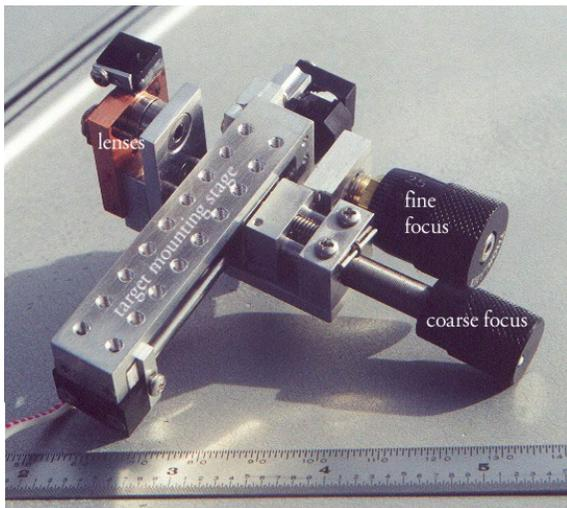
Figure 1. The optical assembly, target mounting stage, and focus mechanism.
