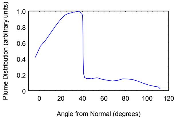
Figure 10. Angular distribution of the plume, parallel to the tape direction.
