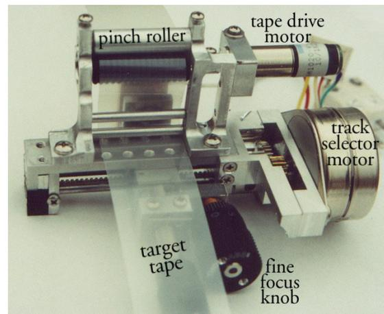
Figure 3. The optical assembly and focusing, track selector and tape drive mechanisms.
