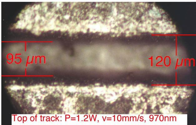
Figure 6. Photomicrograph of continuous burn track.
