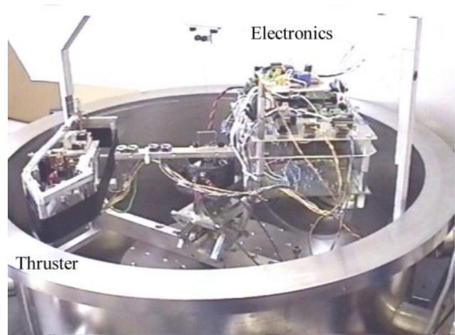
Figure 5. The thruster and electronics mounted on the force test stand inside our vacuum chamber.
