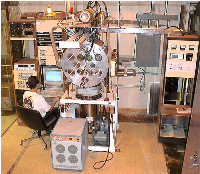
Figure 2 – Vacuum facility for HCMT testing.
