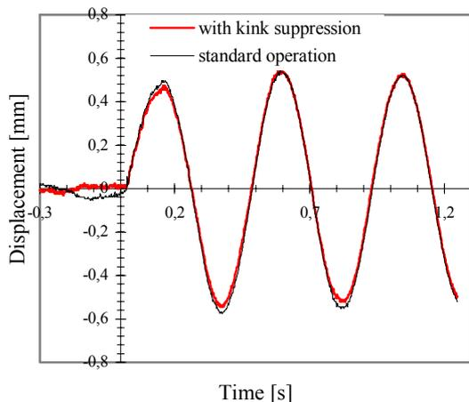
Fig. 7: Mobile mass oscillations with and without plate insertion (mfr=400 mg/s;  $B_{ext} = 40$  mT;  $\Delta V_{PFN} = 1400$  V).
