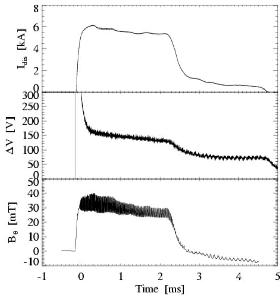
Fig. 2: Time history of a typical discharge: total plasma current  $I_{\text{dis}}$ , applied voltage  $\Delta V$ , and  $B_{\theta}$  measured by one probe of the internal diagnostic system (mfr= 400 mg/s and  $B_{\text{ext}}=100$  mT in this case).
