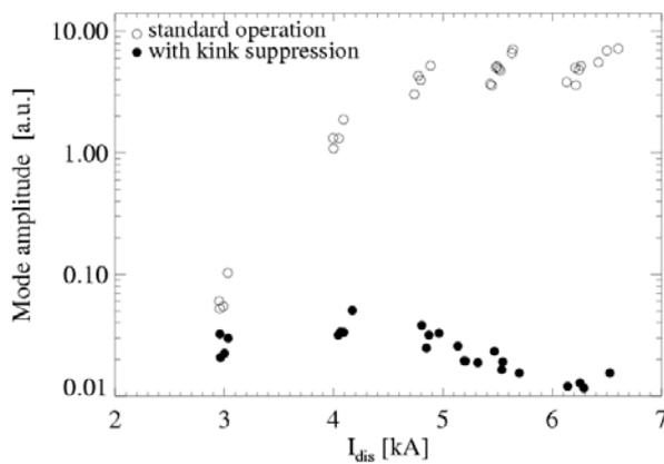
Fig. 5: Mode amplitude plotted as a function of the total plasma current without and with (full circles) effective kink suppression (mfr= 400 mg/s;  $B_{ext} = 40$  mT).
