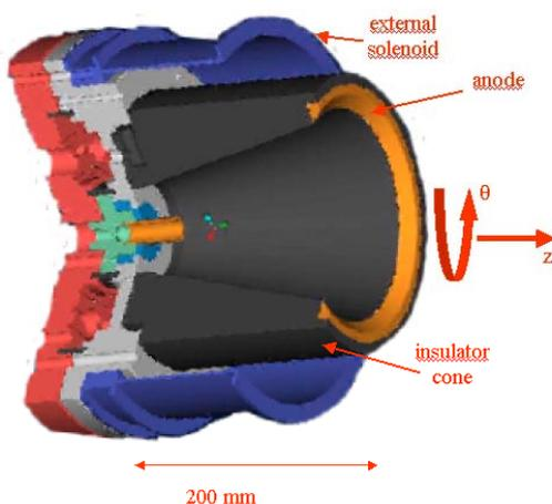
Fig. 1: Schematic of the MPD thruster under investigation, showing anode and cathode shape, and the cylindrical system of coordinates used.
