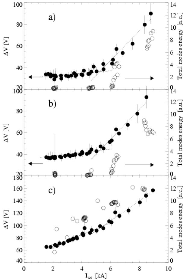
Fig. 3: Applied voltage  $\Delta V$  (full circles) and total mode energy plotted as a function of the plasma current, for three different  $B_{\text{ext}}$  values (from ref. 14).
