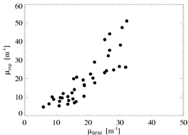
Fig. 9 Experimental  $\mu_{\text{exp}}$  value, plotted as a function of that predicted by the Bessel Function Model  $\mu_{\text{BFM}}$ .
