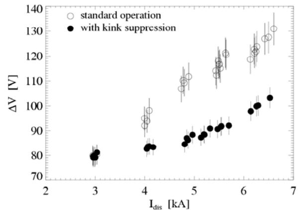
Fig. 6: Applied voltage  $\Delta V$  plotted as a function of the total plasma current without and with (full circles) effective kink suppression (mfr= 400 mg/s;  $B_{ext} = 40$  mT).
