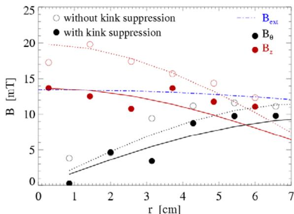
Fig. 10: Experimental radial  $B_\theta$  and  $B_z$  profiles, without and with (full circles) effective kink suppression. Dashed blue line is the radial profile for  $B_{\text{ext}}$  at the thruster outlet.
