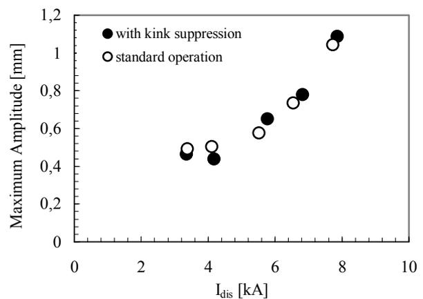
Fig. 8: Maximum amplitude of oscillation of the mobile mass, as a function of the discharge current, with and without plate insertion (mfr= 400 mg/s;  $B_{ext} = 40$  mT).
