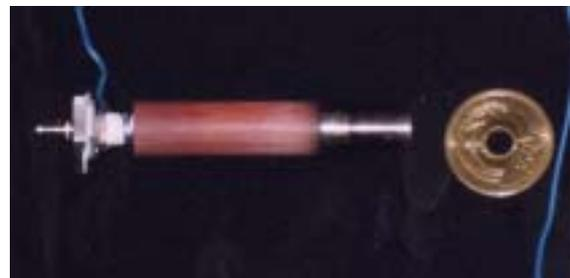
(b) A photo of very low-power gas-propellant plasma-jet microthruster.
