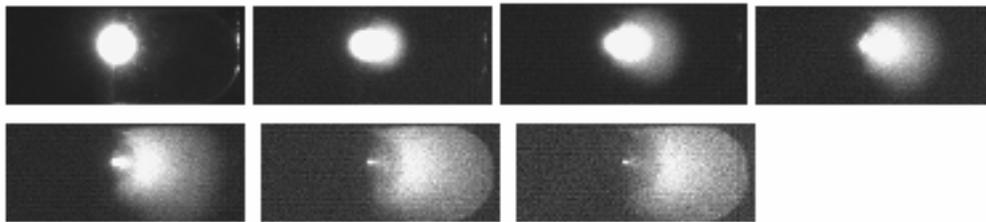
**Figure 1. Plasma without magnetic field (at  $10^{-5}$  Torr cell pressure, YAG 200 mJ/pulse @1064 nm). Frames with time delay (with respect to the laser pulse) ranging from 50 to 750 ns.**
