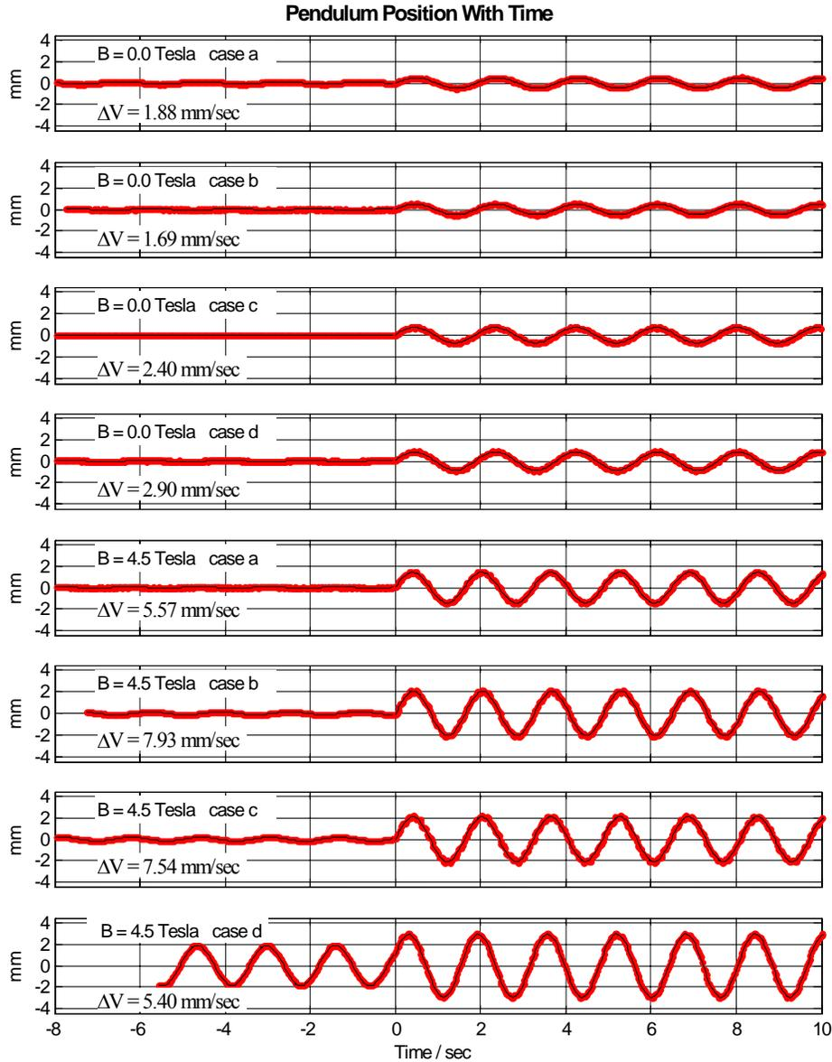
**Figure 3. Pendulum position plotted with time with no applied magnetic field (four cases) and with an applied field of 4.5 Tesla (four cases).**
