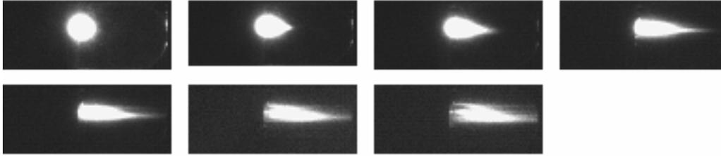
**Figure 2. Plasma with 4.5 Tesla magnetic field along the laser beam (at  $10^{-5}$  Torr cell pressuer, YAG 200 mJ/pulse @1064 nm). Frames with time delay (with respect to the laser pulse) ranging from 50 to 750 ns.**
