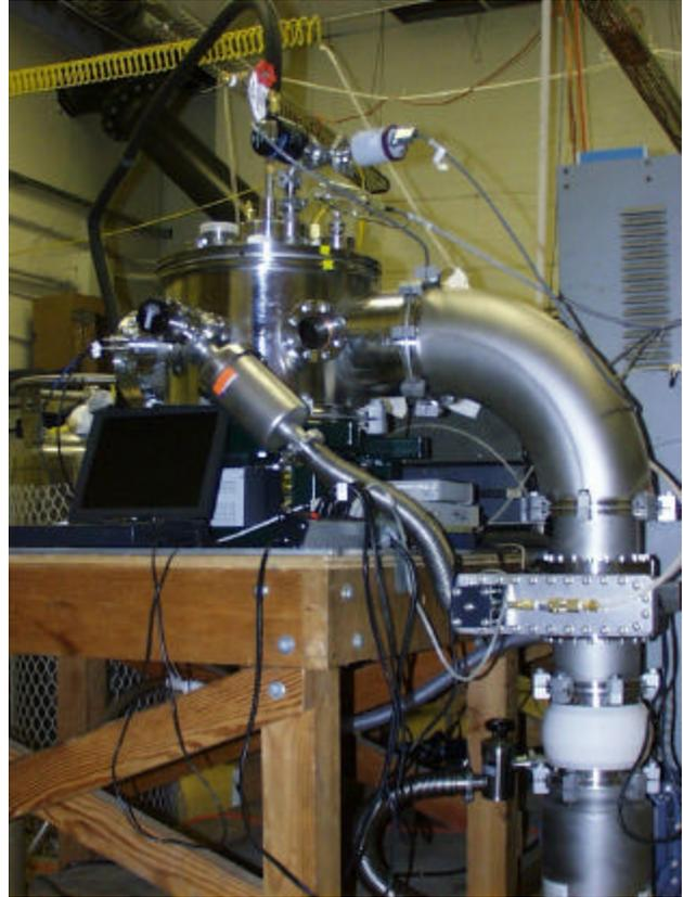
Figure 11 – Vacuum chamber setup.
