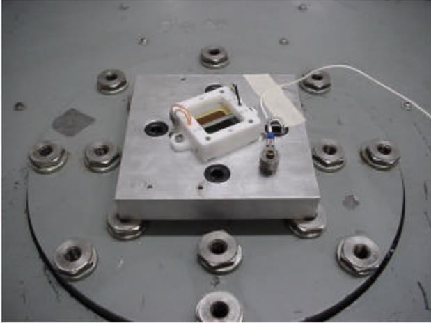
Figure 29 – FMMR EU mounted on the shake table with an aluminum fixture for z-axis random vibration testing.
