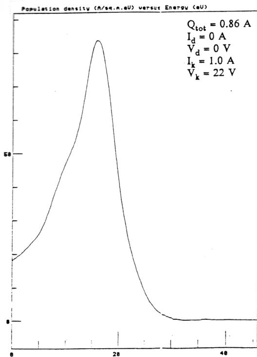
Figure 4 – Ion energy spectrum from Figure 3 (Culham data)<sup>6</sup>.
