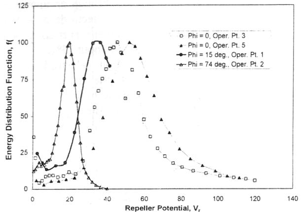
Figure 8 – Ion energy distribution function (Aerospace Corp. data)<sup>4</sup>.
