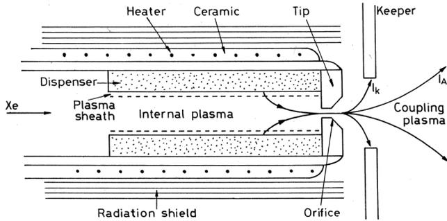
Figure 1 – HC/keeper assembly (QinetiQ).
