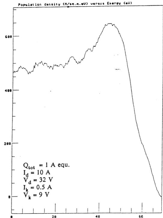
Figure 6 – Ion energy spectrum at 1 A eq. current and 10 A discharge current (Culham data)<sup>6</sup>.
