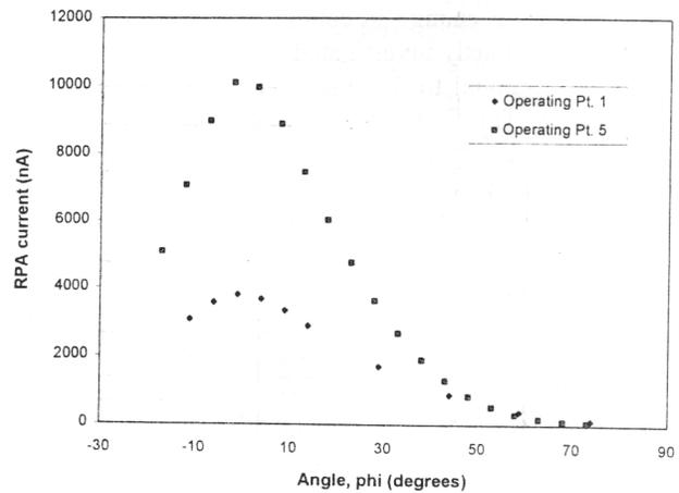
Figure 2 – Angular distribution of ion efflux (Aerospace Corp. data)<sup>4</sup>.
