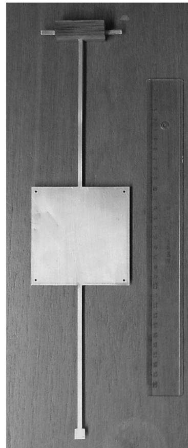
Figure 11 – Aluminum target and insulating mount (ruler is 30 cm).
