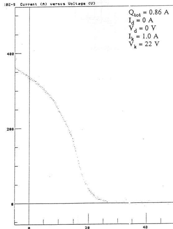
Figure 3 – RPA trace at 0.86 A eq. Current (Culham data)<sup>6</sup>.
