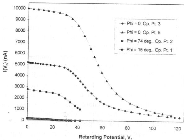
Figure 7 – RPA current vs. retarding potential (Aerospace Corp. data)<sup>4</sup>.
