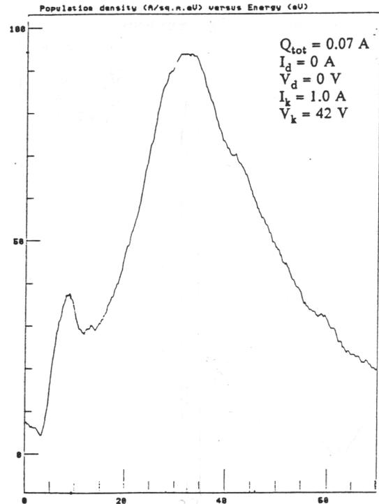
Figure 5 – Ion energy spectrum at 0.07 A eq. current and 1.0 keeper current (Culham data)<sup>6</sup>.
