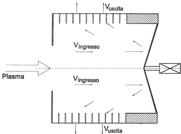
Figure 10 – Cylindrical target section and operation<sup>57</sup>.
