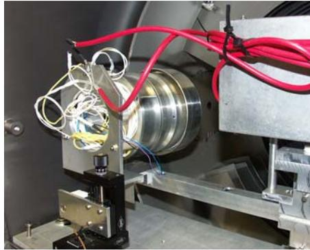
**Figure 8. Cluster Module mounted on the balance**
