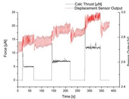
**Figure 7. Example of raw data from thrust measurement**
