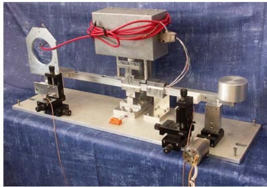
**Figure 1. ARC-sr  $\mu\text{N}$  thrust balance**
