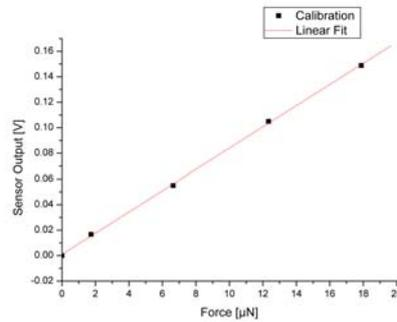
**Figure 6. Single emitter calibration data**
