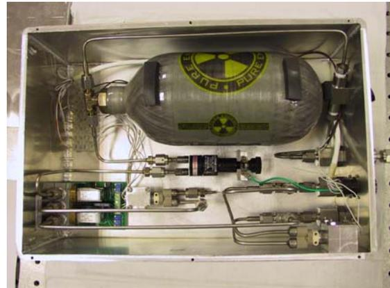
**Figure 9. Gas Pressurized feed system electronics and argon supply tank.**
