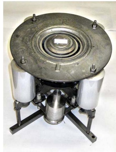
Figure 5. Refurbished D160 lab model 2-stage hall thruster<sup>12</sup>.
