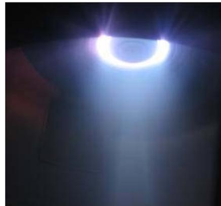
Figure 6. D160 2-stage TAL operating at 3kV in TsNIIMASH test facility.
