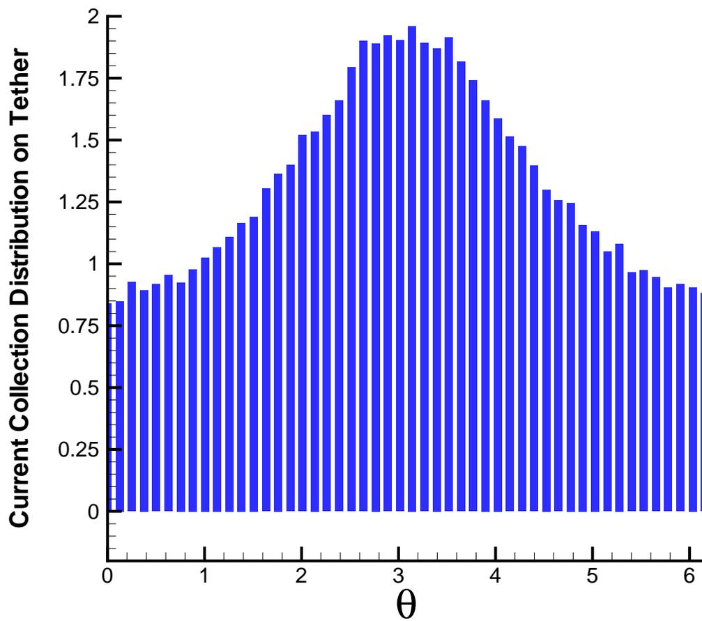
Figure 2: The distribution of electron current collection on the tether surface.  $\theta$ (rad.) is taken from the wake side and increases counterclockwise.
