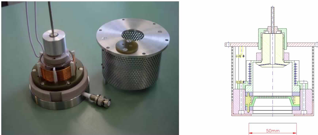
Fig. 3. photo and drawing true to scale and of the 4-cm \mu NRIT-4 prototype
