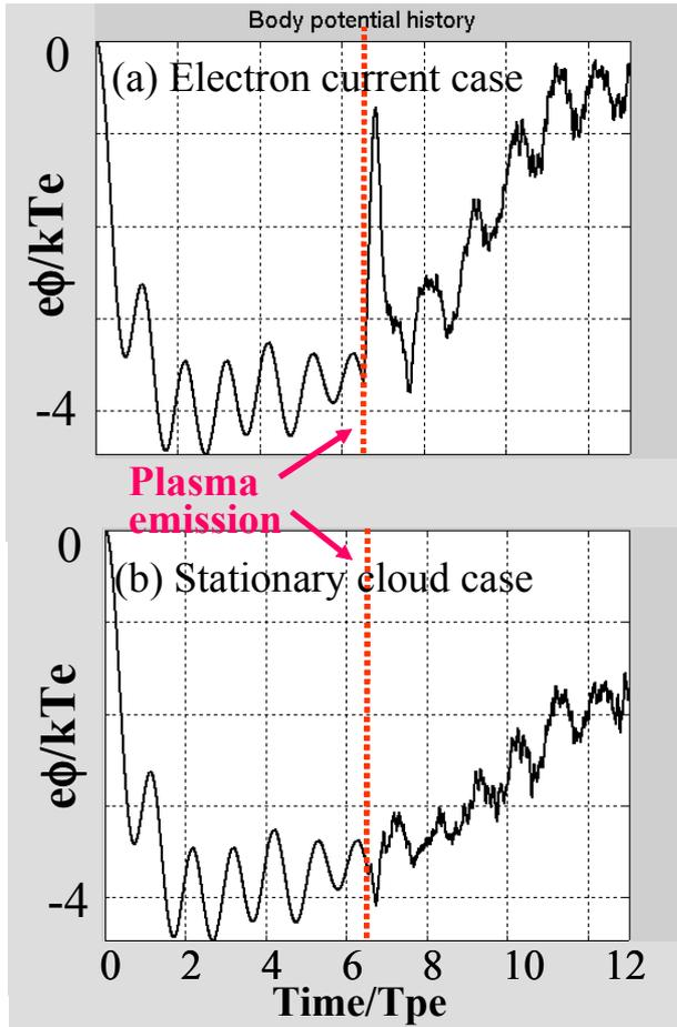
Figure 3 – Temporal variation of the body potential for (a) electron current model and (b) stationary plasma cloud model.
