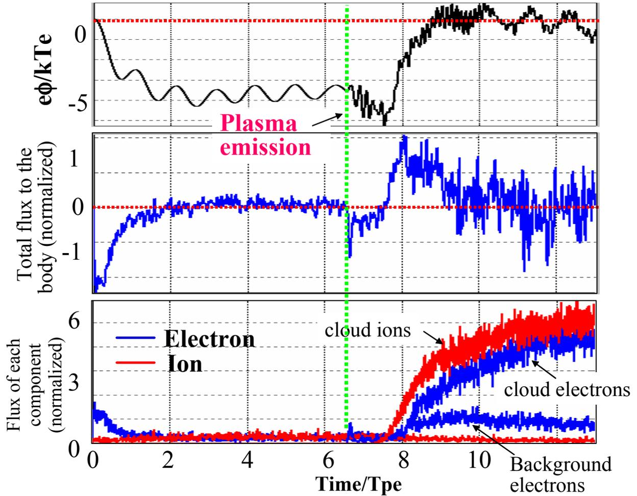
Figure 2 – Temporal evolution of the body potential (top), total flux to the body (middle), and flux of each plasma component to the body (bottom). The physical quantities in the panels are normalized.
