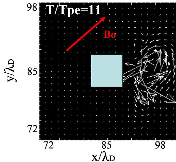
Figure 6 – Snapshot of current density profiles. Each arrow represents current density at each grid point in the vicinity of the body.
