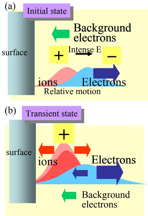
Figure 5 – Schematic illustrations showing (a) initial and (b) transient states of emitted plasma distribution in the electron current model.
