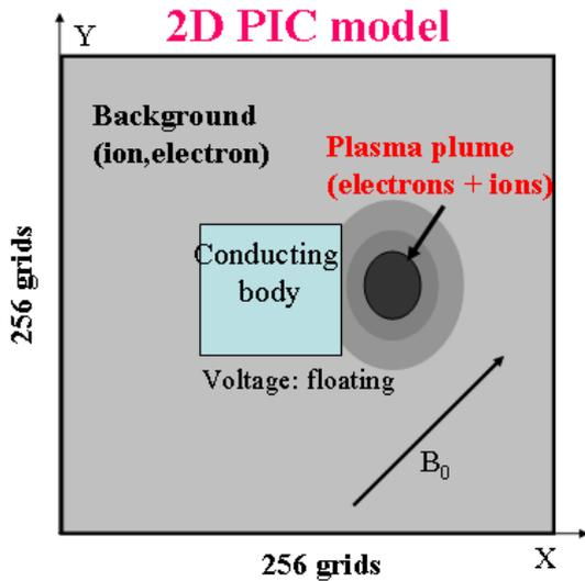
Figure 1 – 2D PIC simulation model
