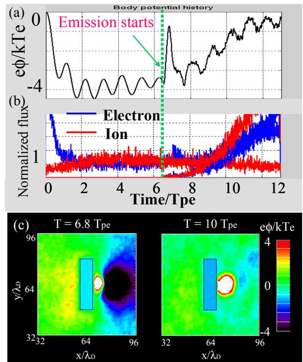
Figure 4 – Temporal evolution of the body potential (top), flux of each component to the body, and (c) snapshots of potential profile in the x-y plane. Rectangular in the potential profile represents the location of the conducting body.
