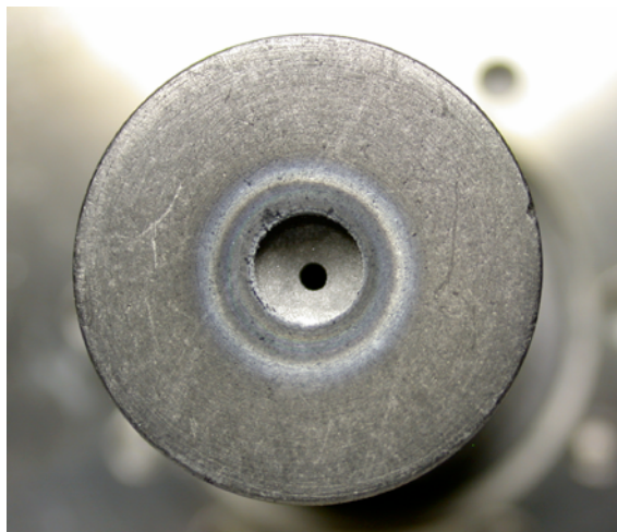
Figure 6. Graphite keeper face discoloration showing ion bombardment pattern for approximately 20 hours of operation at TH15.
