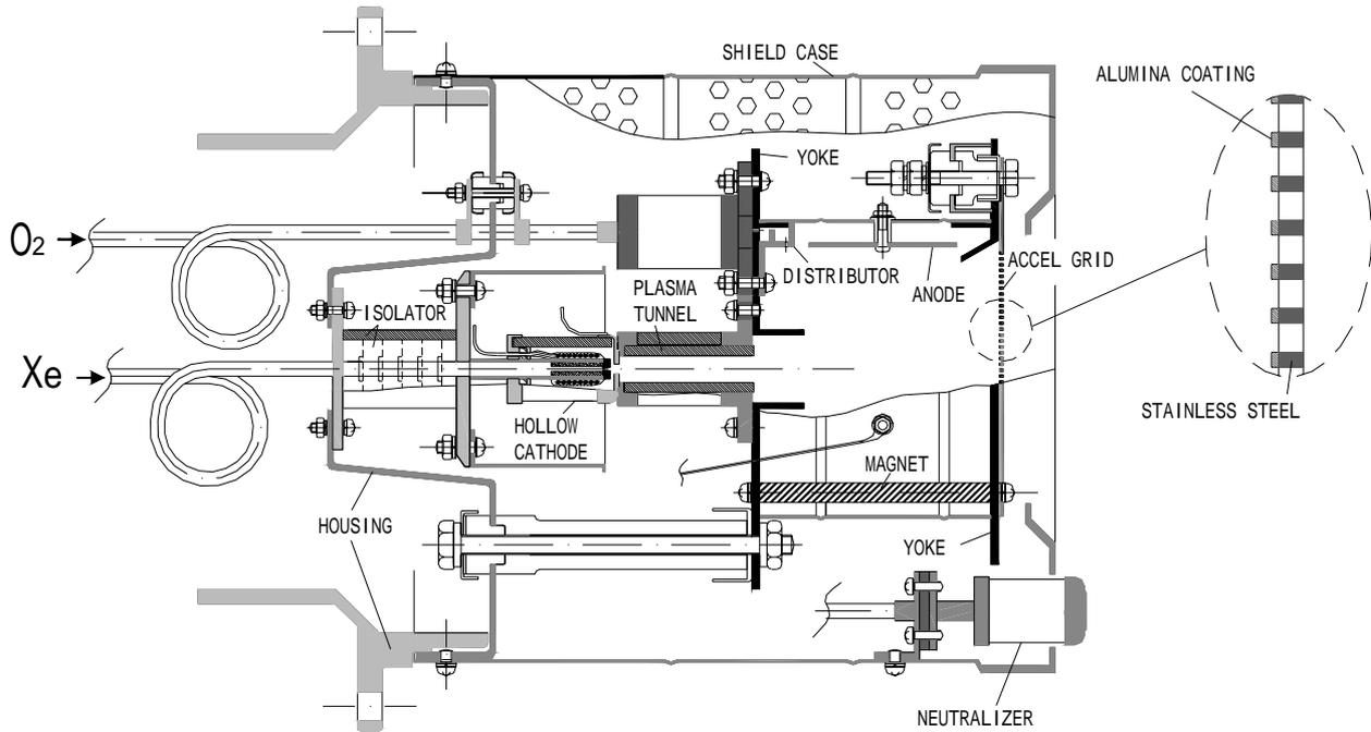
Fig. 2 The oxygen ion thruster configuration with a plasma tunnel ( a long and small diameter tube ) to protect a hollow cathode from oxygen.
