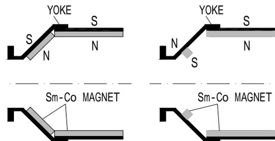
(a) Long magnets of the same polarity. (b) Short magnets of opposite polarity. Fig. 6. Magnets arranged on the conical wall.
