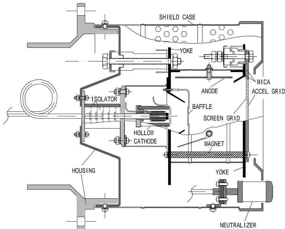
Fig. 1 The PreEM of ETS-III ion thruster ( without mercury tank and vaporizer ) operated by using inert gases.
