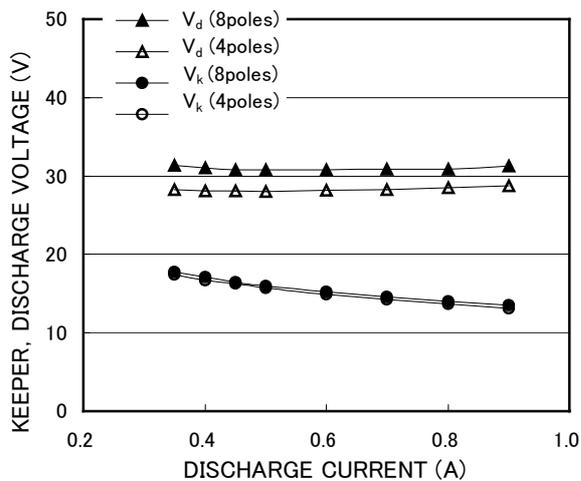
(a) Xe flow rate = 0.3 sccm,  $J_k = 0.2$  A
