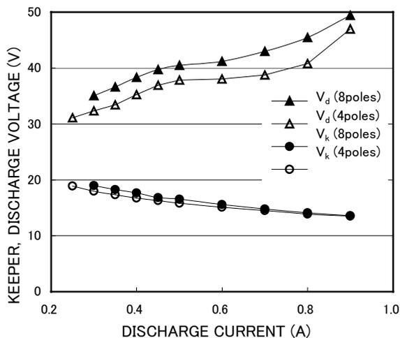
(b) Xe flow rate = 0.2 sccm,  $J_k = 0.2$  A
