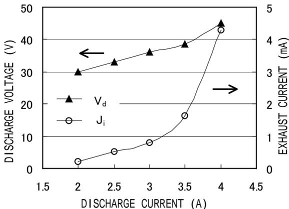
Fig. 4. The discharge voltage and exhaust ion current vs. discharge current by using oxygen. Hollow cathode Xe flow rate = 0.3 sccm Main Discharge  $O_2$  flow rate = 0.9 sccm
