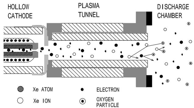
Fig. 3 Functions of the plasma tunnel.
