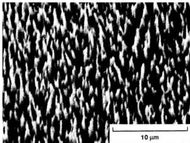
Figure 2a – Typical surface structure of the ion beam textured pyrolytic graphite. The structure is composed of sharp spires with heights and spacings of 6  $\mu\text{m}$  to 12  $\mu\text{m}$  and 3  $\mu\text{m}$  to 6  $\mu\text{m}$ , respectively.
