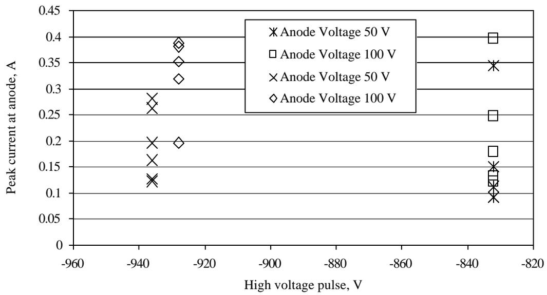
Figure 8 - Initial results of ferroelectric cathode experiments. Electron emission currents measured at the anode for various levels of anode voltage and high-voltage-pulse amplitude.
