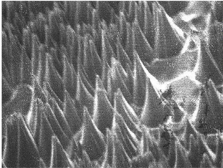
Figure 2b – Typical surface structure of the ion beam textured copper. The structure is composed of cones with heights and bases of 15  $\mu\text{m}$  to 20  $\mu\text{m}$  and 10  $\mu\text{m}$  to 15  $\mu\text{m}$ , respectively.
