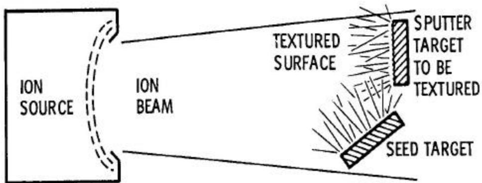
Figure 1b – Illustration of texturing of the copper coupons using “tantalum seed texturing”.
