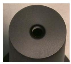
Figure 19. Post-Test Photograph of Discharge Cathode Assembly Keeper Orifice Plate.
