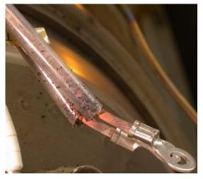
Figure 17. Post-Test Inspection Photograph of Wire Harness Near Discharge Cathode Assembly. Note decomposition of wire insulation inside the intact Teflon sleeving.
