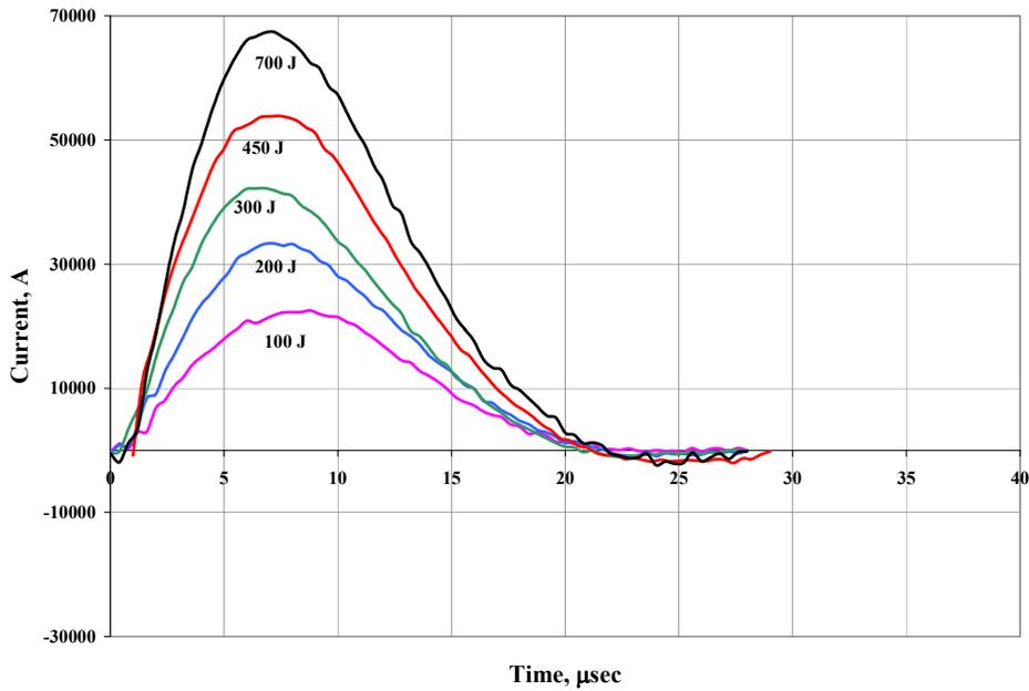
Figure 8. Discharge current waveforms for *HEPPT2* for a thruster capacitance of 260  $\mu\text{F}$ .
