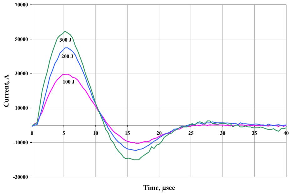
Figure 6. Discharge current waveforms for *HEPPT2* for a thruster capacitance of 100  $\mu\text{F}$ .
