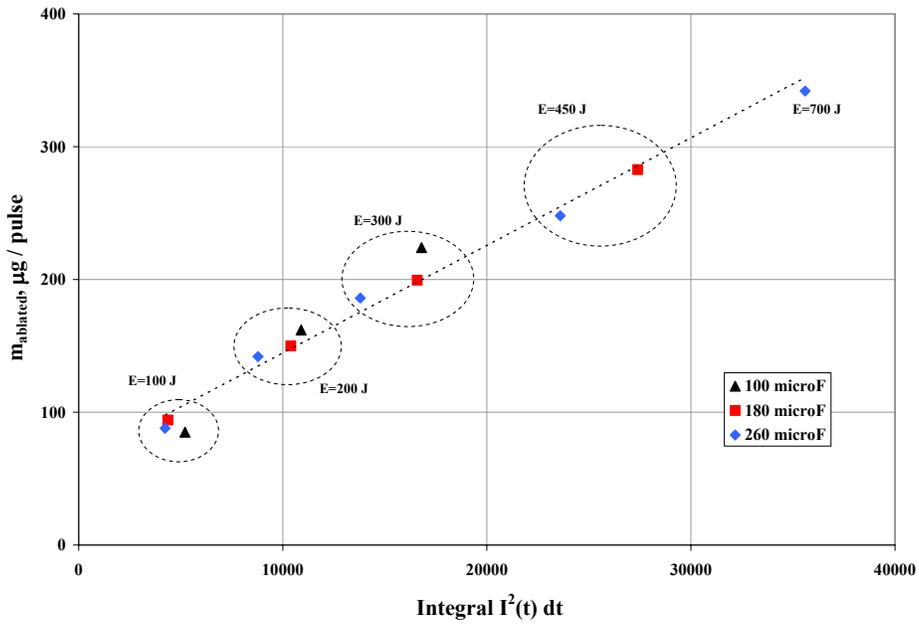
Figure 13. PTFE ablated mass vs.  $\int I^2(t) dt$  for discharge energy levels between 100 J and 700 J.
