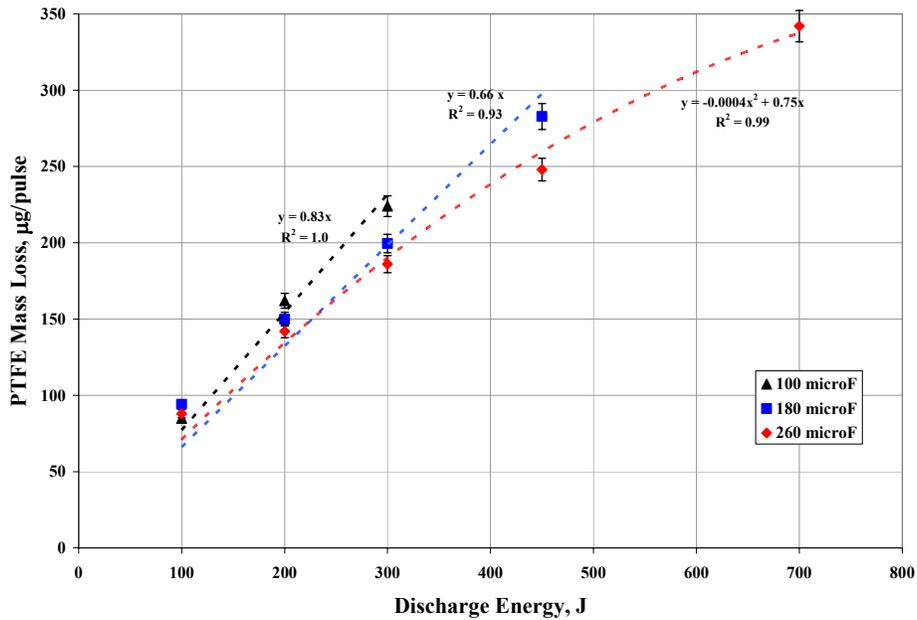
Figure 9. *HEPPT2* PTFE mass loss magnitudes for discharge energy levels between 100 J and 700 J.
