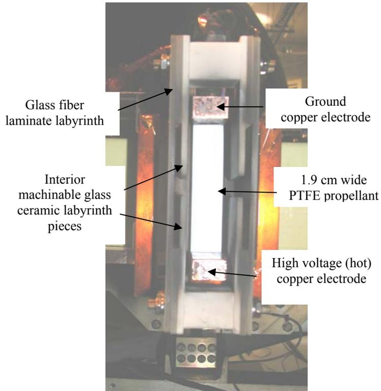
Figure 2. Picture of the inter-electrode region of *HEPPT2*.
