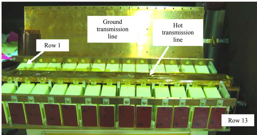
**Figure 1. Picture of partially disassembled *HEPPT2* showing the 13 rows of capacitors.**
