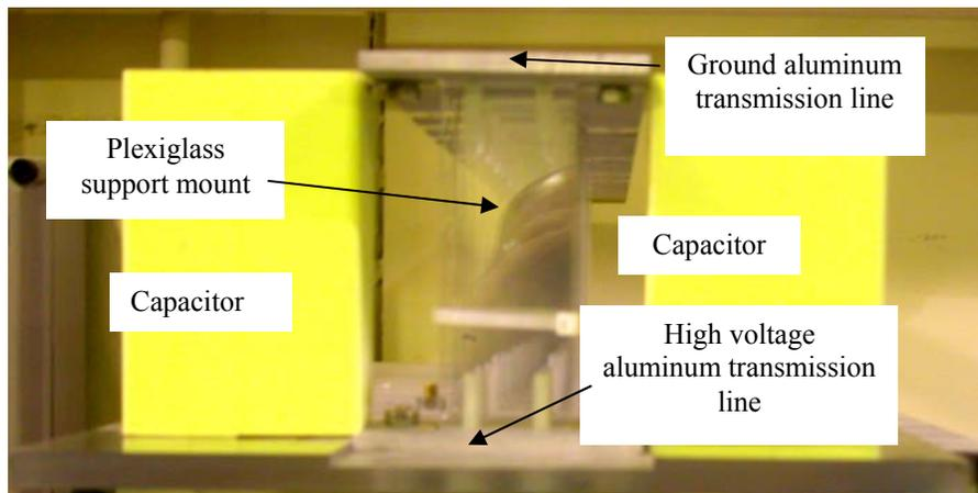
Figure 3. Backview picture of *HEPPT1b* showing the ground and hot transmission lines, capacitors, and plexiglass supporting mount.
