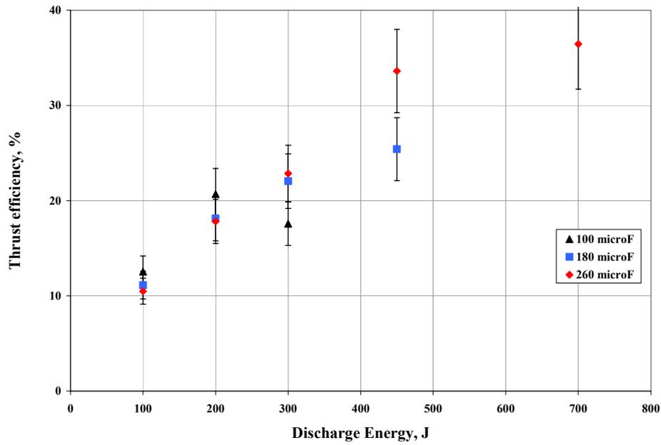
Figure 12. *HEPPT2* thrust efficiency magnitudes for discharge energy levels between 100 J and 700 J.
