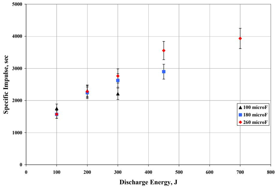
Figure 11. *HEPPT2* specific impulse magnitudes for discharge energy levels between 100 J and 700 J.
