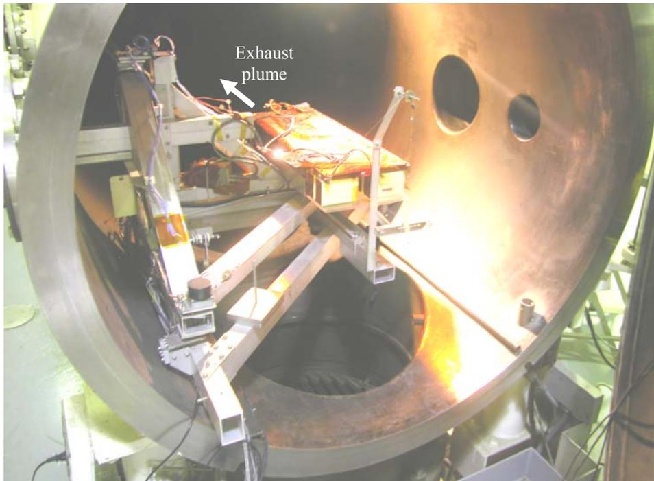
Figure 5. Picture of *HEPPT2* mounted on the PPT thrust stand in VF-3 at NASA GRC.
