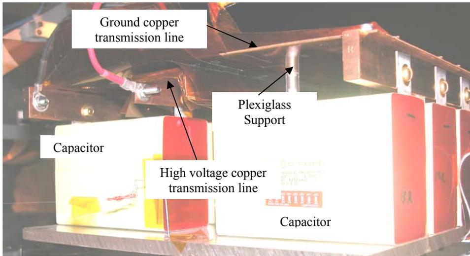
Figure 4. Backview picture of *HEPPT2* showing the copper transmission lines, capacitors, and plexiglass supporting mounts.
