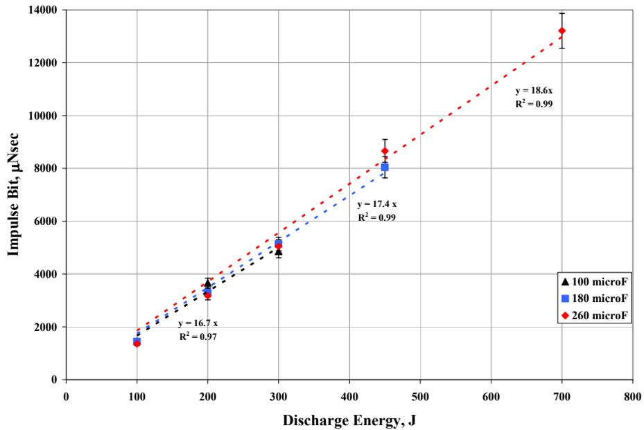
Figure 10. *HEPPT2* impulse-bit magnitudes for discharge energy levels between 100 J and 700 J.
