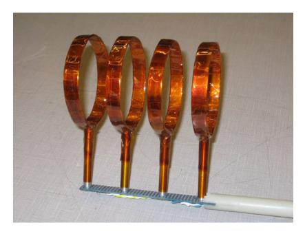
Figure 4. Photograph of the loop antenna showing its four aluminum rings. The rings are insulated from the plasma by wrapping them in Kapton tape.
