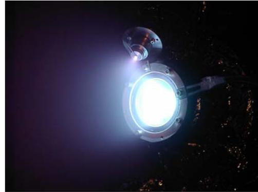
Figure 12. HEMP 3050 DM8 thruster in operation with neutraliser HKN 5000
