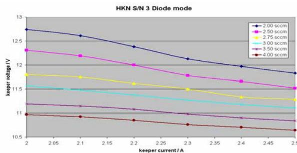
Figure 7. Neutraliser HKN 5000 BB1 performance in the diode mode. Keeper voltage vs current
