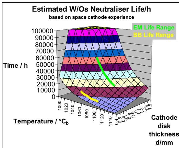
Figure 4. Neutraliser ignition life estimation as function of cathode disk temperature and thickness
