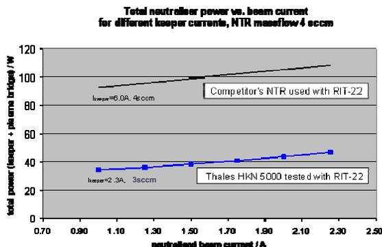
Figure 14. Total neutraliser power consumption of the Thales HKN 5000 and a competitive design
