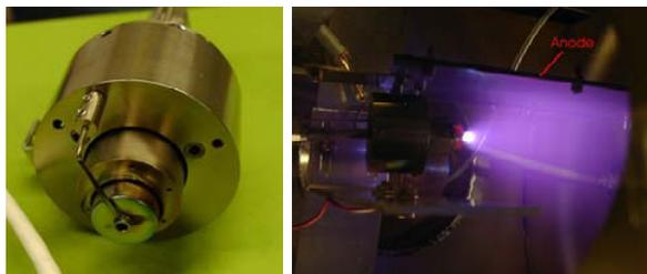
Figure 6. Neutraliser HKN 5000 BB (left), operating in triode mode in vacuum (right)
