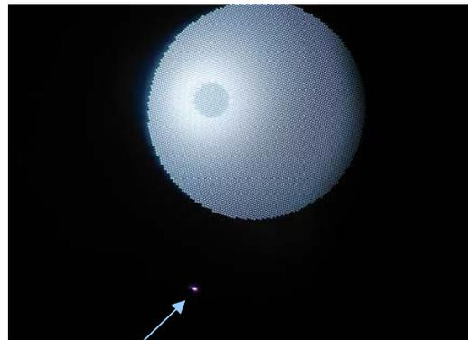
Figure 13 a, b. BB2 model of the HKN 5000 neutraliser mounted to RIT 22
