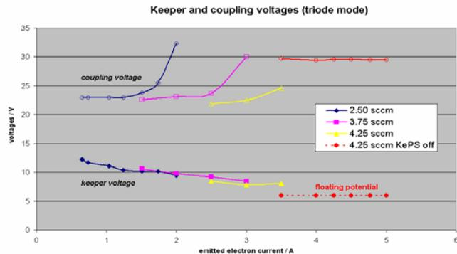
**Figure 8. Neutraliser HKN 5000 BB1 performance in the triode mode. Keeper and coupling voltage vs emitted electron (anode) current.**
