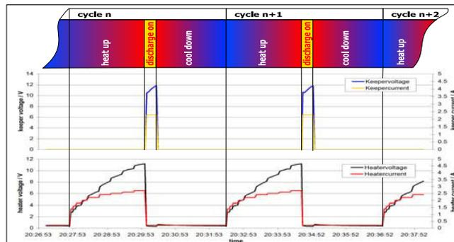
**Figure 10. Three out of totally 4500 ignition cycles in diode mode of HKN 5000 BB1 neutraliser**
