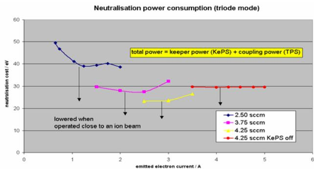
**Figure 9. Neutralisation cost vs anode current of HKN 5000 BB1 neutraliser in triode mode.**
