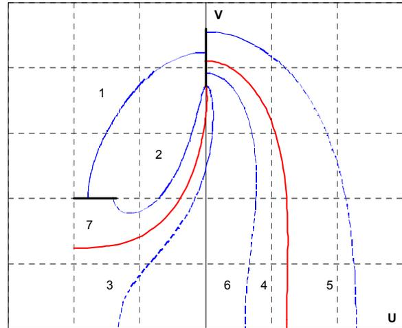
Fig.5. Typical configuration of lines of force for modern Hall thruster magnet system.
