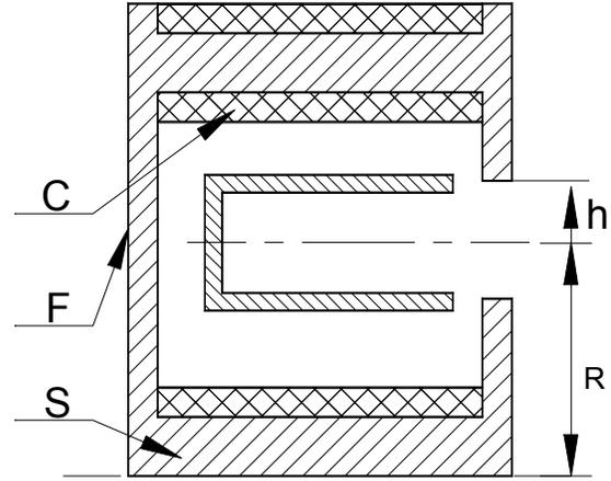
Fig1. Configuration of Hall thruster magnet system.
