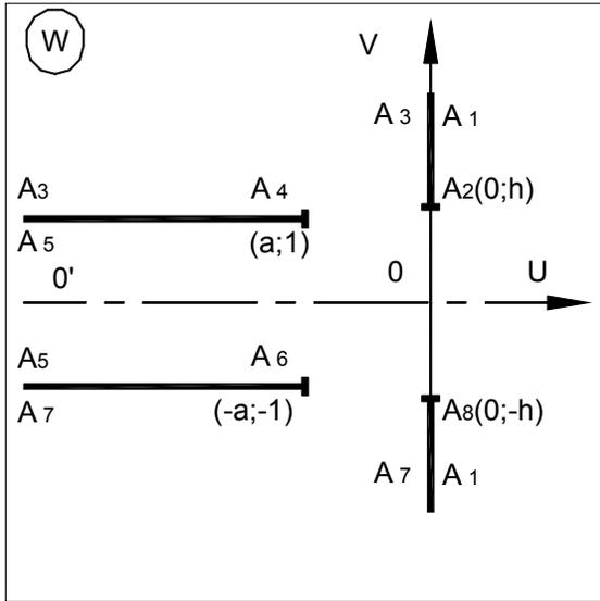
Fig.2 Idealized configuration of magnet system in discharge area.
