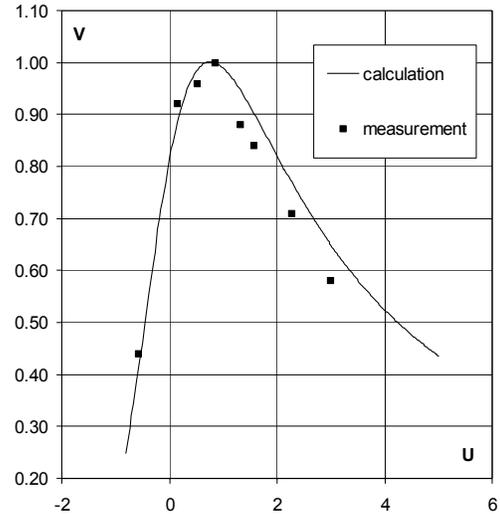
Fig.6 Comparison of calculated and measured values of magnetic field along axis of symmetry.
