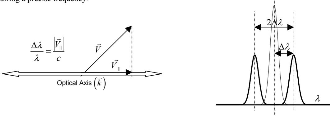
**Figure 4. Left: Schematic of velocity vector, CRDS optical axis (wave vector points both directions), and velocity vector parallel to optical axis. Right: Measured CRDS lineshape (thick line) has both up- and down-shifted peaks. The separation of the shifted peaks,  $2\Delta\lambda$ , gives the parallel velocity component. The unshifted lineshape is shown with a thin line.**
