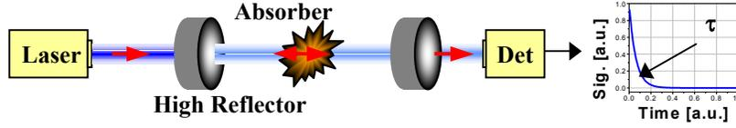
**Figure 1. Schematic diagram of cavity ring-down spectroscopy (CRDS). Laser light is coupled into a high reflectivity cavity where it bounces back and forth many times. A detector behind the cavity measures the decay of the light intensity inside the cavity, which may be related to the concentration of the absorbing species.**
