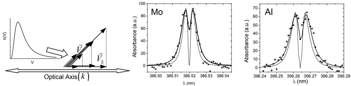
**Figure 5. Left: Schematic representation of CRDS optical axis with multiple unidirectional velocity vectors oriented at  $45^\circ$ , and projections on optical axis. Middle/Right: Velocity measurements for Mo and Al. Symbols - measured lineshape; Thick line – model fit; Thin line – model fit without laser convolution.**
