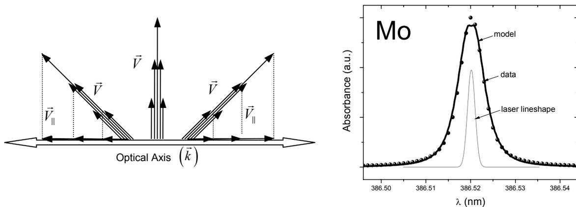
**Figure 6. Left: Schematic representation of CRDS optical axis with multiple velocity vectors of differing directions and magnitudes, and projections on the optical axis. Right: Velocity measurement for Mo.**
