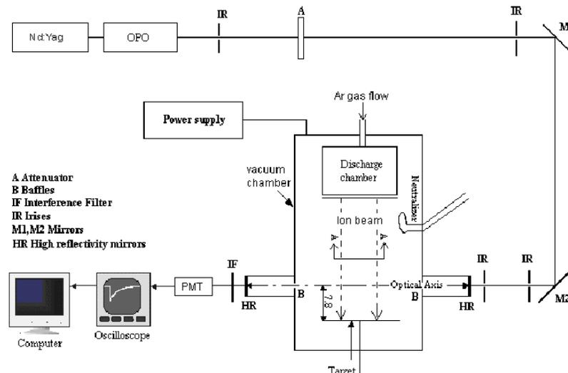
**Figure 2. Schematic diagram of sputtering apparatus and CRDS system. The ion beam is normally incident upon the target and optical axis is located 7.8 cm upstream of the target. The ring-down cavity has a length of 0.75 m, and uses 0.5-m radius of curvature mirrors. An OPO laser system is used as the light source, and a photomultiplier tube (PMT) detects the light exiting the cavity.**
