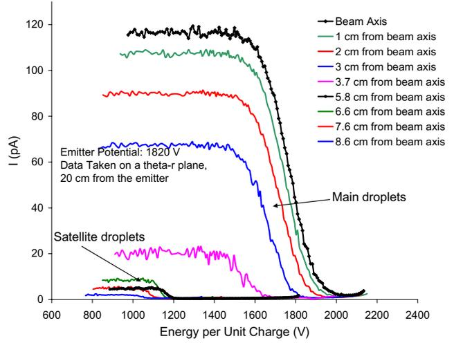
**Figure 2. Retarding potential spectra of a 87 nA PC/EMI-Im electro spray, taken at different polar angles.**
