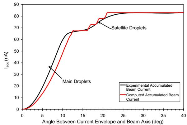
Figure 9. Computed and measured accumulated current versus polar angle .
