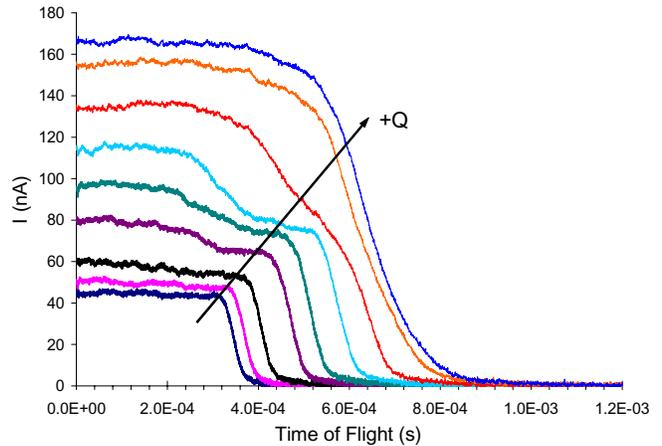
Figure 1. Time of flight spectra of PC/EMI-Im electrospray beams.
