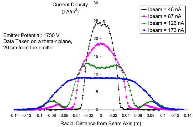
Figure 4. Beam profiles for different beam currents.
