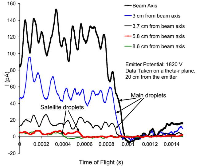
**Figure 3. Time of flight spectra of a 87 nA PC/EMI-Im electro spray, taken at different polar angles.**
