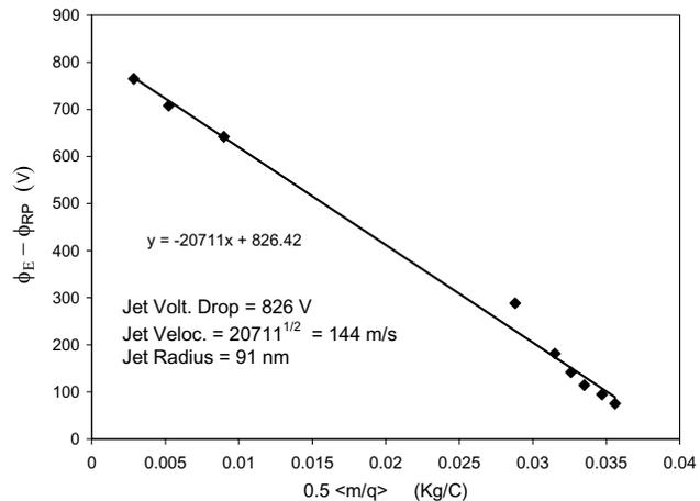
Figure 6. Estimation of droplet initial velocity and potential. Note that the y-axis displays the emitter voltage (1820 V) minus the droplet retarding potential.
