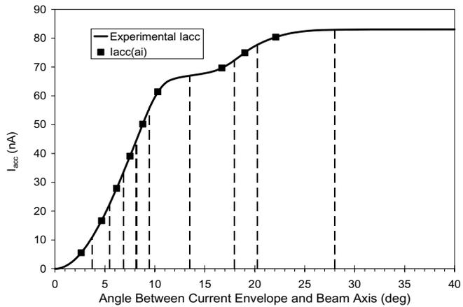
Figure 5. Accumulated beam current versus polar angle for  $I_B = 87$  nA.
