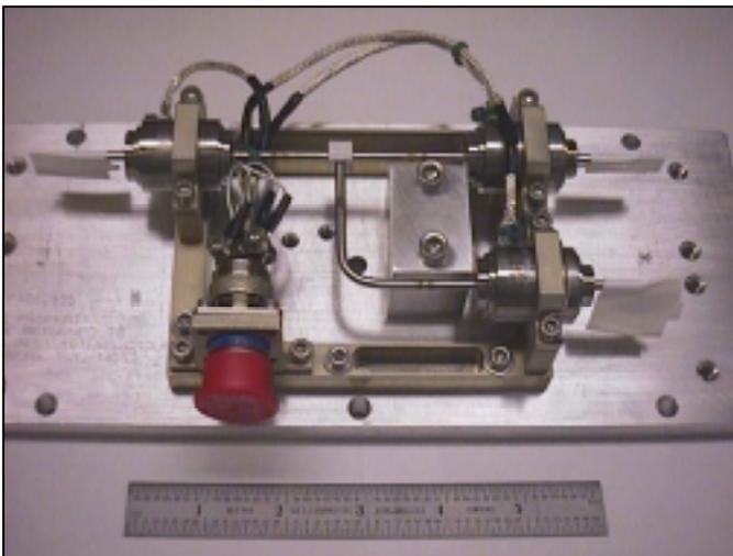
Figure 1. The XFC provides proportional flow control of xenon gas in a small, lightweight package
