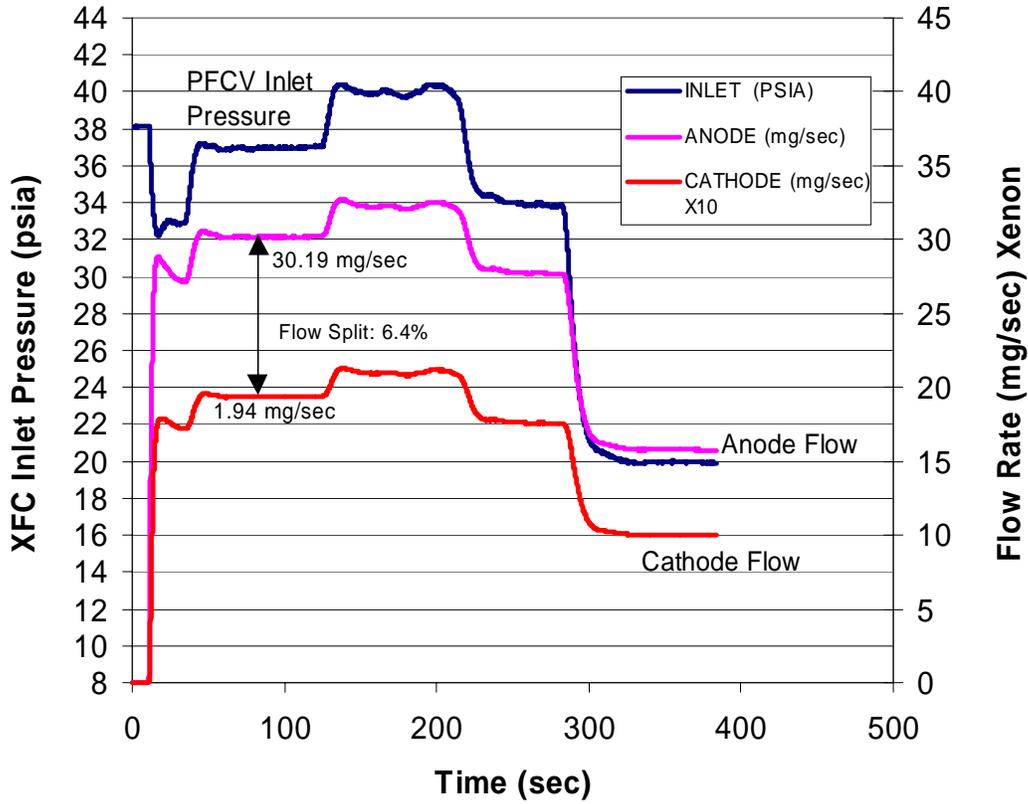
Figure 5. A flow split of 6.4% to 6.5% was achieved with the ground test XFC over an XFC inlet pressure range of 34 to 40 psia. Note that the flow rate of the cathode valve is shown ten times the actual flow rate.
