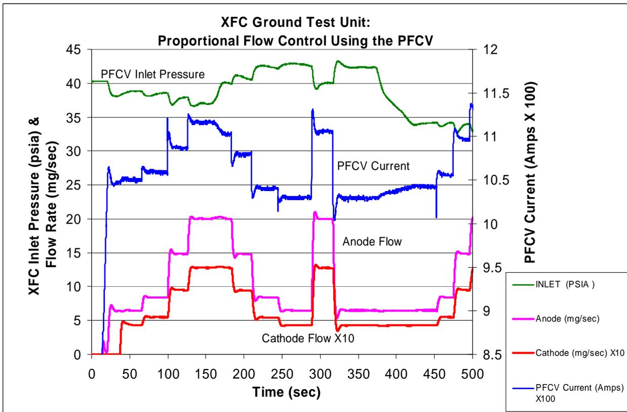
Figure 6. Proportional control of the xenon flow using closed loop feedback to control the input current to the PFCV based on the flow rate through the anode solenoid valve. Note that the flow rate through the cathode valve is shown ten times the actual flow rate.
