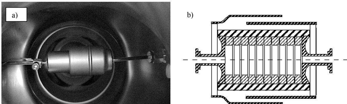
Figure 1. a) Image of device in test chamber and b) sketch of isolator
