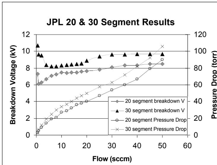
Figure 9. Voltage hold-off of the 20 and 30-segment isolator as a function of xenon flow rate.
