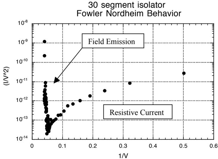
Figure 5. *Fowler-Nordheim Plot for the 30-segment isolator under high vacuum conditions*
