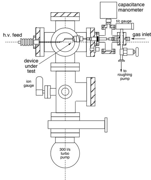
Figure 2. *Schematic Layout of Vacuum Chamber Test Arrangement*
