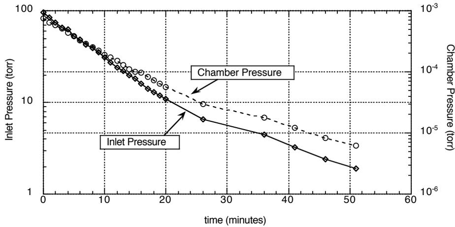
Figure 3. Chamber pressure as a function of time following pressurizing the inlet chamber to 100 torr of nitrogen
