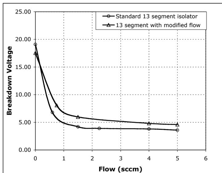
Figure 11. Paschen curve for the standard 13-segment isolator and one with modified flow.
