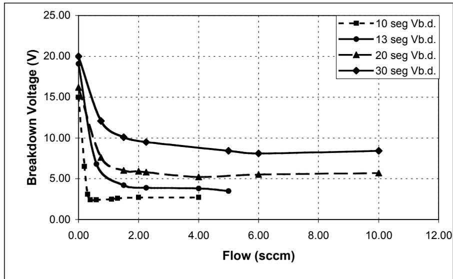
Figure 7. Breakdown voltage as a function of inlet pressure for 10, 13, 20 and 30 segment propellant isolators. For 20 and 30 segment devices a small upswing in voltage at 10 sccm is indicated.
