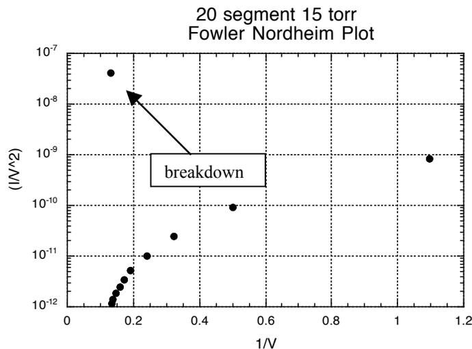
Figure 6. *Fowler-Nordheim Plot for the 20-segment isolator with flow. Inlet pressure was set to 15 torr.*
