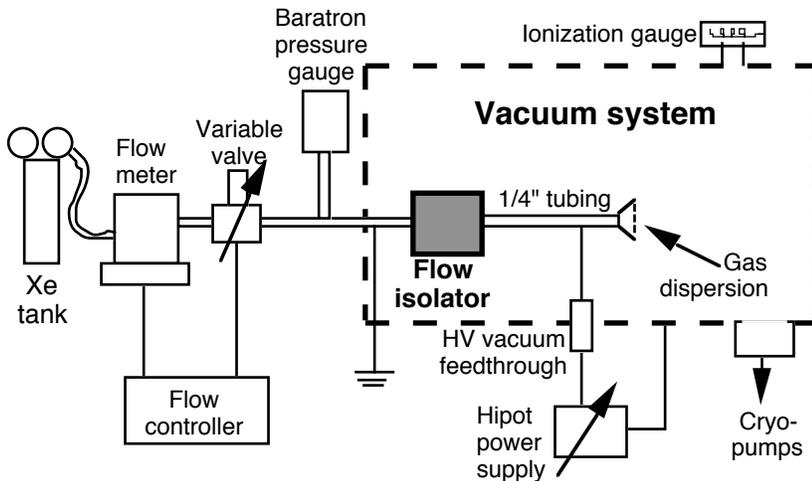
Figure 8. Schematic of the flow isolator tests at JPL.
