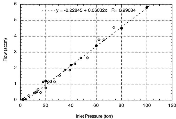
Figure 4. Determination of xenon gas flow rate for a given inlet gas pressure. Squares indicate flow calculated from the size of the flow orifice, diamonds represent measured values based on the known pumping speed and chamber volume.
