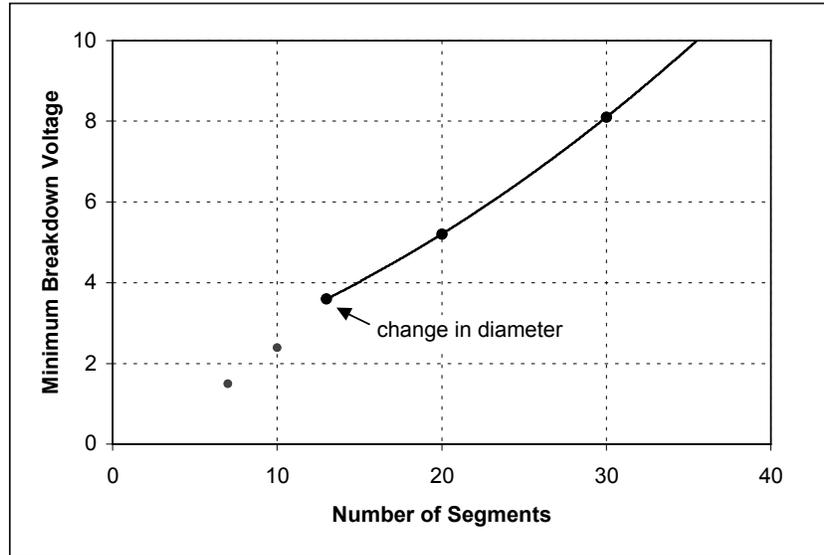
Figure 10. Breakdown voltage versus number of segments for L-3 ETI gas flow isolators
