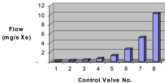
**Figure 7: Valve Flow Rates**
