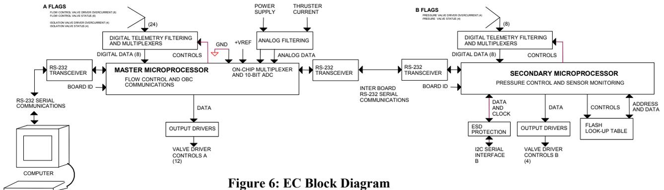
Figure 6: EC Block Diagram
