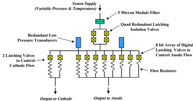
**Figure 13: Flight XFS Block Diagram**
