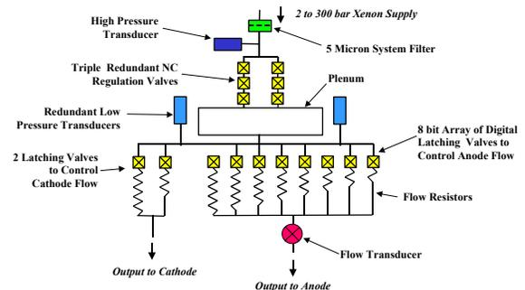
**Figure 11: Flight PCM Block Diagram**
