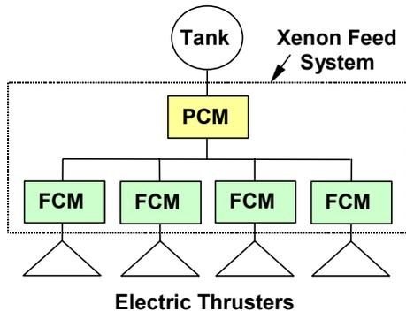
**Figure 1: Xenon Feed System (XFS)**
