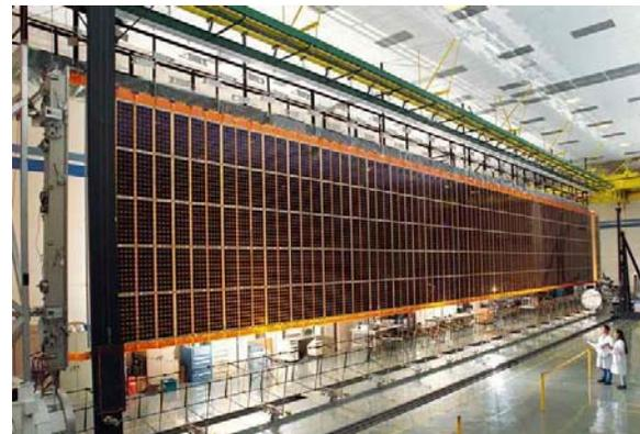
**Figure 14 ISS solar array being tested at LMSS, Sunnyvale**
