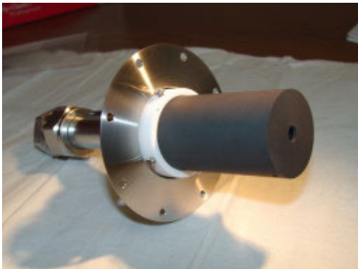
Figure 7. Pretest photograph taken of the lab model hollow cathode assembly with graphite keeper.
