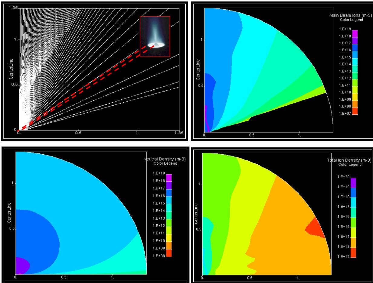
Figure 7. Results of 2-D plume simulation of SPT100 showing ion trajectories (top left), main-beam ion density (top right), neutral density (bottom left) and total ion density (bottom right).
