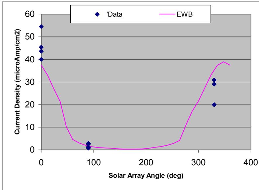
Figure 9. Comparisons of EWB calculation (solid line), incorporating the results from the 2-D plume code, with ion-flux measurements from the DRT1 sensor onboard Express A#3 during rotation of the solar arrays.
