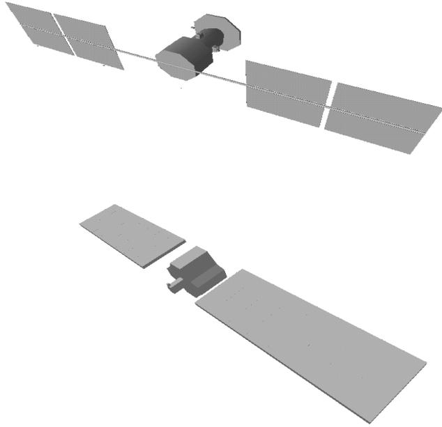
Figure 4. EWB models of EXPRESS (top) and DS-1 (bottom) used to assess HET-Array interactions.
