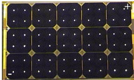
Figure 15. International Space Station array coupon showing 15 8cm x 8cm cells.
