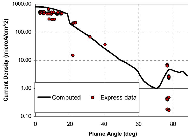
Figure 10. Comparisons between 2-D plume simulations and Express-A ion-flux data (scaled down to 1-m).
