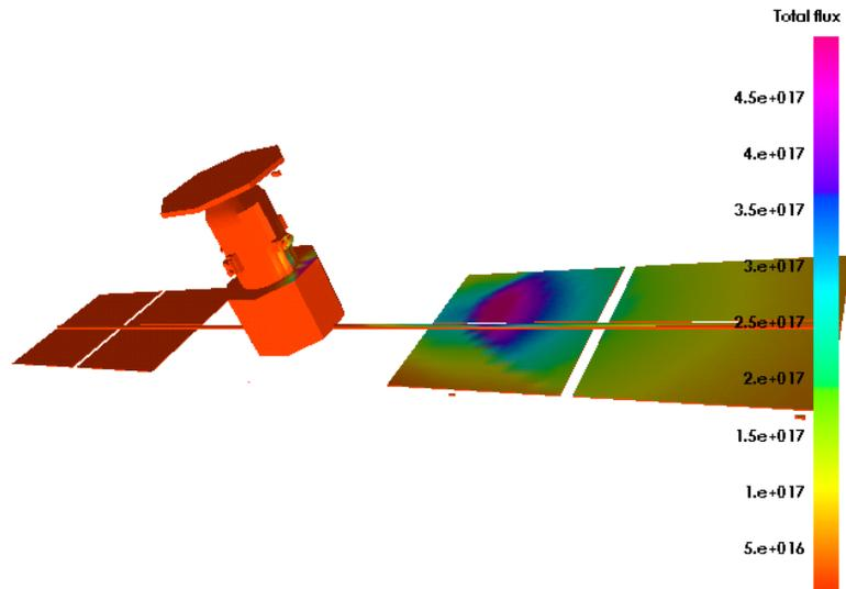
Figure 12. EWB calculation of the flux of ions to the EXPRESS array during operation of the RT4 SPT-100 thruster (flux is given in  $1/s\cdot m^2$ ).
