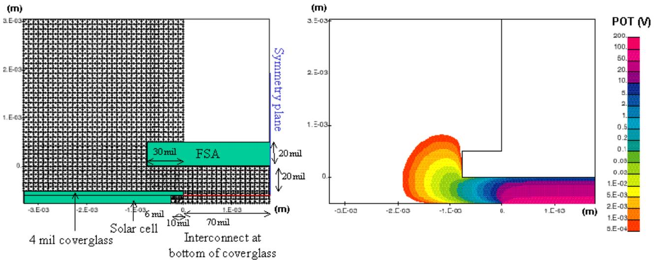
Figure 13. 2-D, solar array modeling will be used to scale plasma interactions, such as current collection, to the higher densities not attainable in the chamber. (Left: Front Side Aperture and solar array geometry and computational region. Right: computed potential profile).
