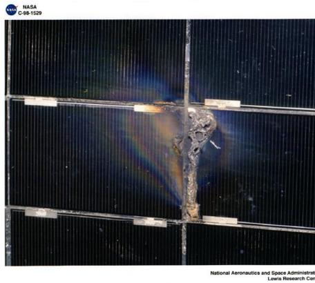
Figure 1. Permanent arc damage to a Terra array coupon during preflight tests.
