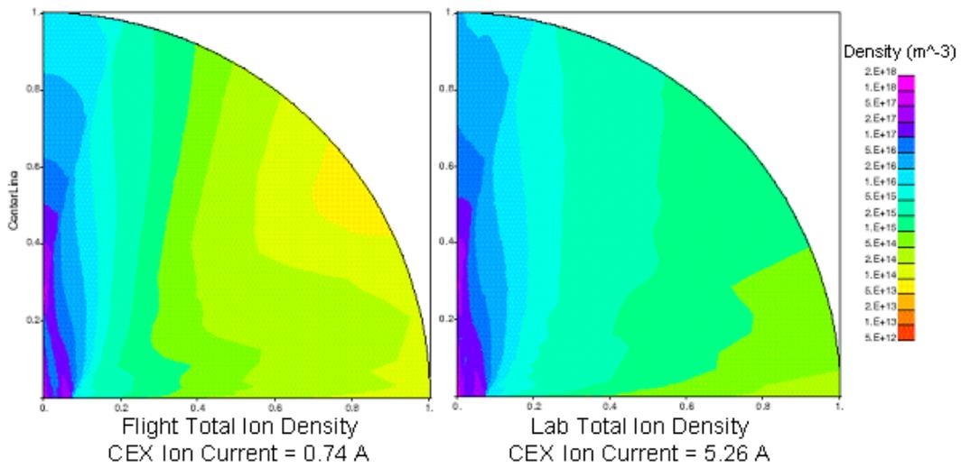
Figure 8. HET plume maps for lab and space conditions showing dominance of background density in the charge-exchange plume production.
