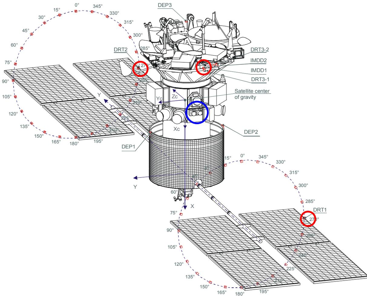
Figure 5. Location of ion-flux sensors (DRT) and SPT100 unit on the Express-A3 Satellite.
