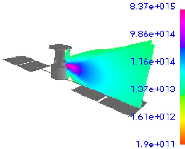
Figure 11. EWB calculation of the density in the vicinity of the EXPRESS arrays during operation of RT4 SPT-100 thruster (density is given in  $m^{-3}$ ).
