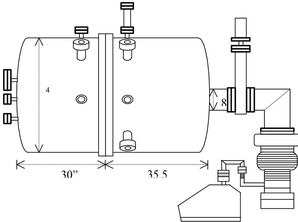
Figure 14. MSFC vacuum chamber to be used for plasma testing of candidate array designs.
