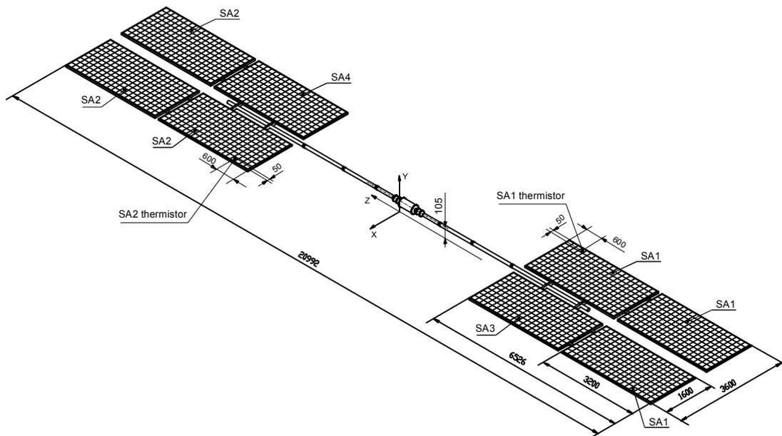
Figure 3. The Express-A solar array (showing location of temperature sensors).
