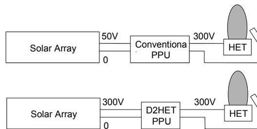
Figure 2. D2HET's high voltage solar arrays result in a smaller, lighter, simpler, PPU.
