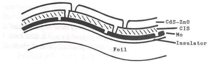
Structure of a flexible CIS submodule.
