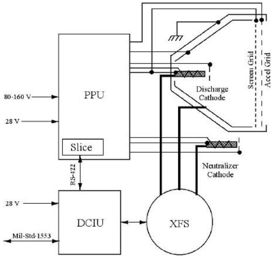
Figure 1. Simplified Ion Propulsion System Block Diagram
