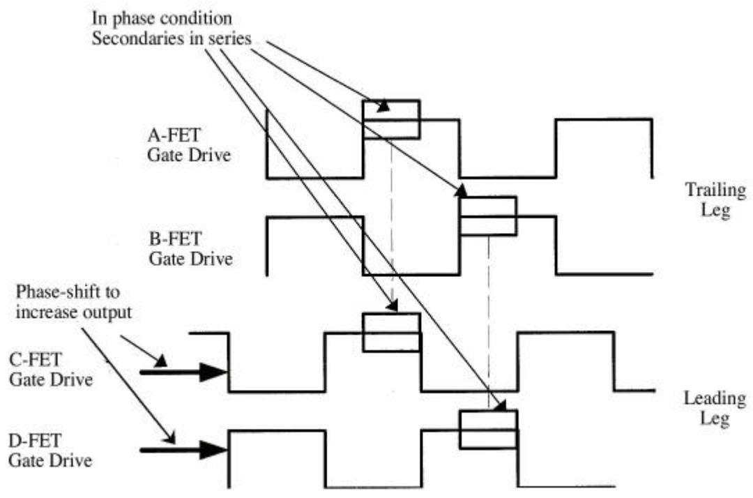
Figure 4. Phase-Shift Modulation Gate Drives
