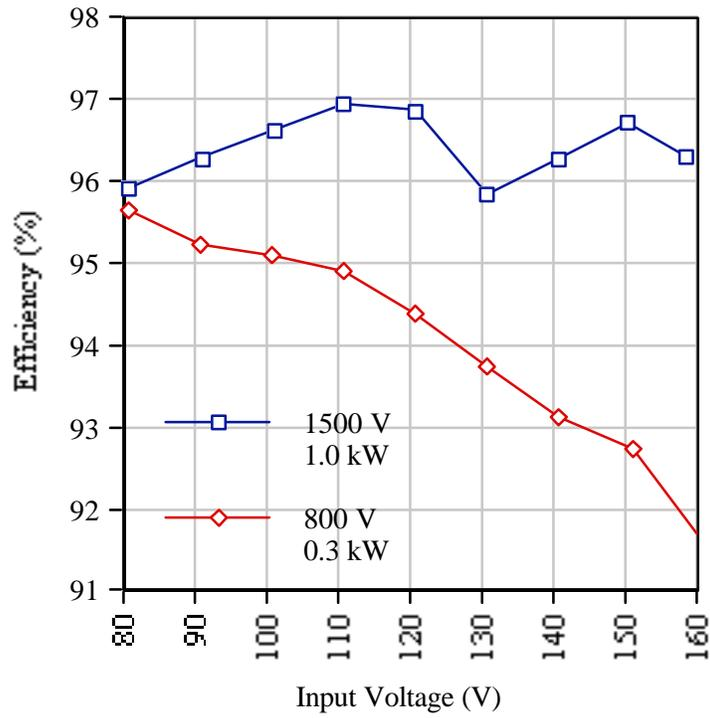
Figure 9. Beam Power Module Efficiency vs. Input Voltage
