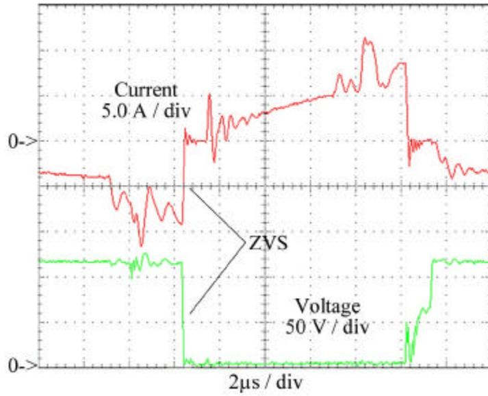
Figure 7. Zero-Voltage-Switching Waveforms
