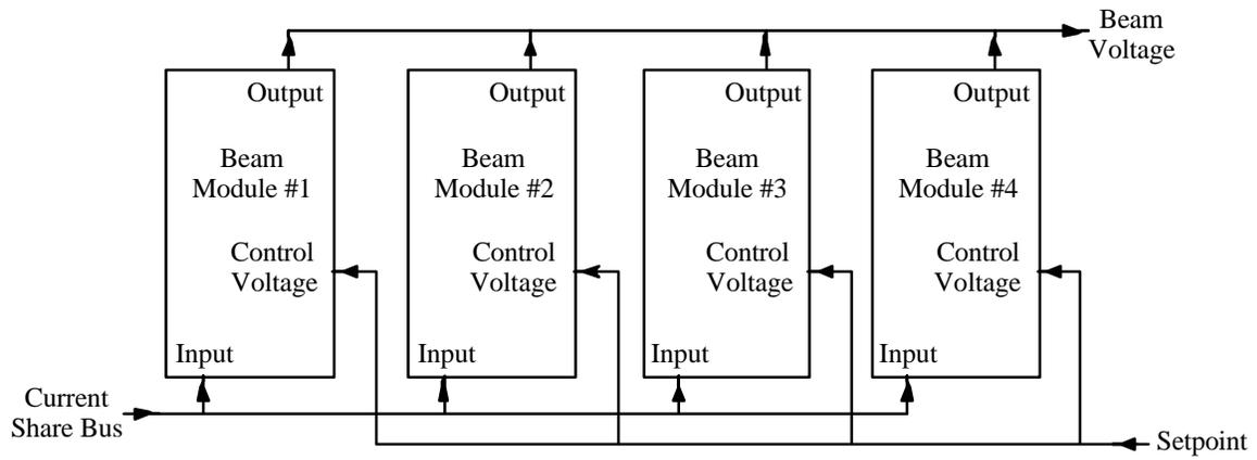
Figure 8. 5 kW Modular Beam Supply Block Diagram
