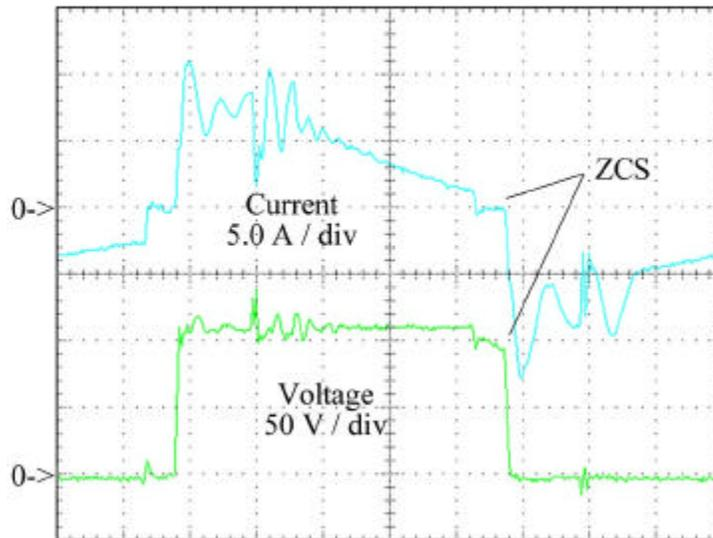
Figure 6. Zero-Current-Switching Waveforms
