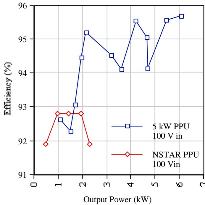
Figure 10. Estimated 5 kW PPU Efficiency vs. Output Power
