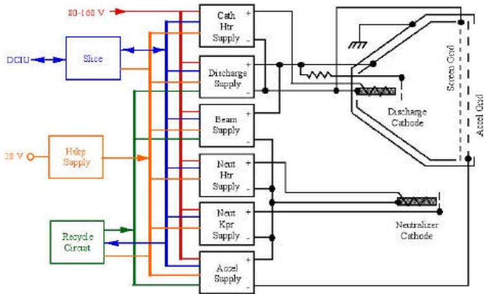
Figure 2. Simplified Power Processing Unit Block Diagram
