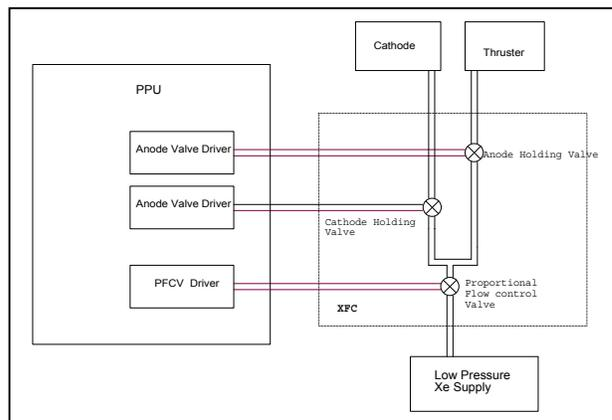
Figure 2 - Xenon Flow Control (XFC) and Valve Drivers
