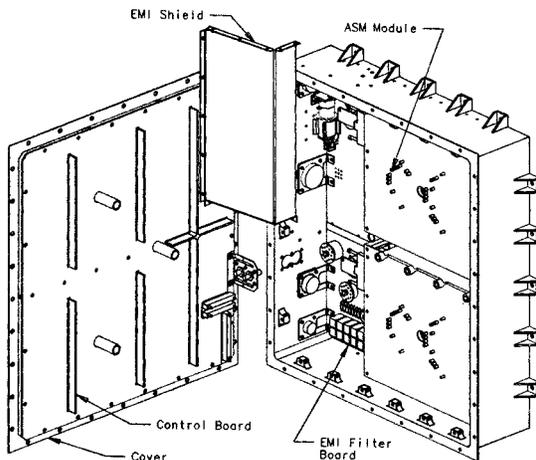
Figure 4 - HTPS PPU Mechanical Design Overview
