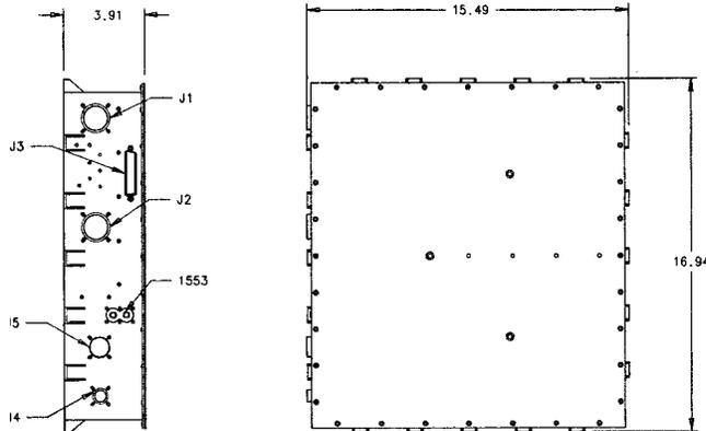
Figure 3 - HTPS PPU Envelope Dimensions
