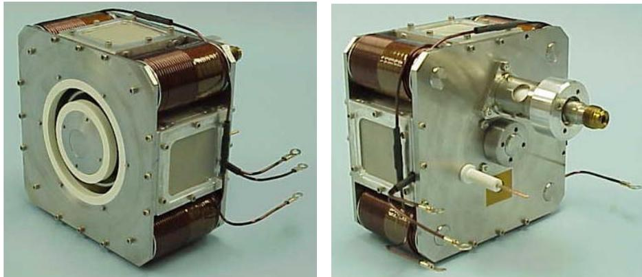
Figure 1 Photographs of the thruster designed and constructed for high  $I_{sp}$  development
