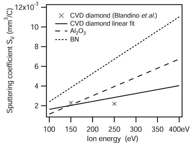
Figure 1- Sputtering coefficients for insulator materials of interest [10, 11].
