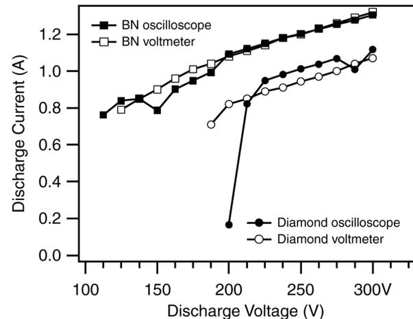
Figure 7 - Comparison of mean current-voltage characteristics for diamond and BN walls, measured with both a digital oscilloscope (black symbols) and a digital voltmeter (open symbols).
