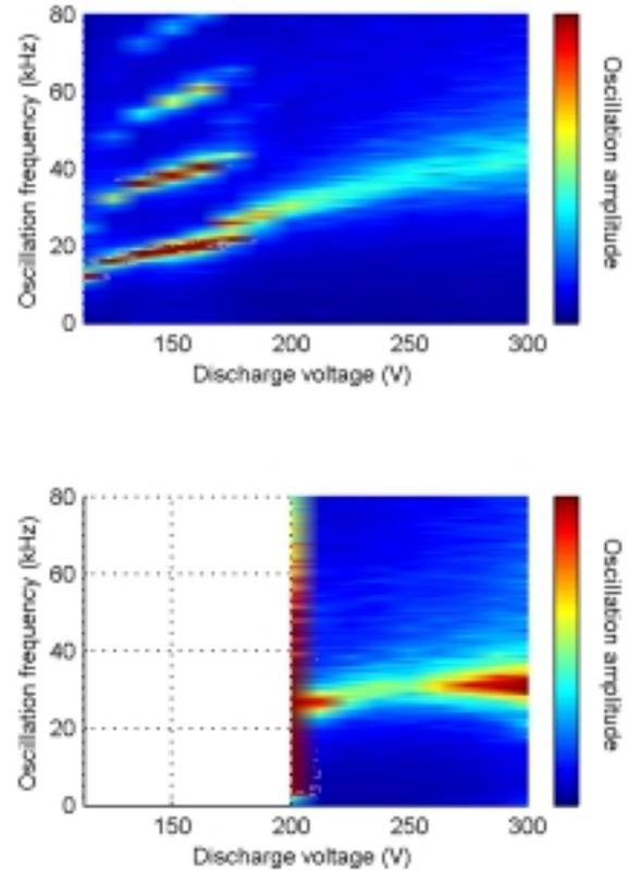
Figure 10 - Current oscillation spectra for the case of a BN channel (top) and for the diamond channel thruster (bottom).
