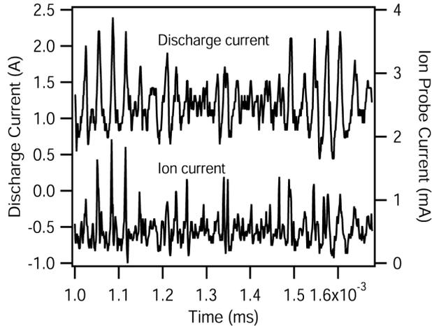
Figure 8 - Sample waveforms recorded for the BN thruster with probe located at the center of the channel ( $x = 0, y = 0$ ).
