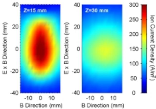
Figure 11 - Mean ion current profiles for BN thruster.
