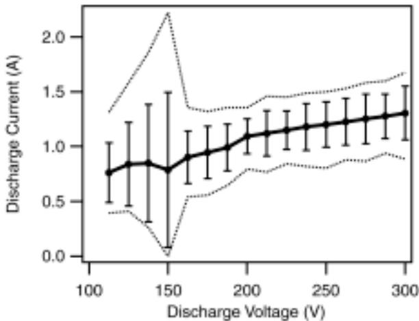
Figure 5-Current-voltage characteristic and oscillation amplitudes of linear Hall thruster with BN walls. Error bars indicate the standard deviation of the oscillating current. Dotted lines are plotted at the top tenth and bottom tenth of the current oscillation range.
