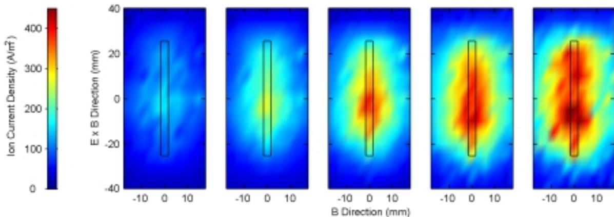
Figure 9 - Breathing oscillation “movie” for BN thruster at 200 V operation.
