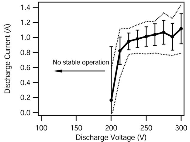
Figure 6- Current-voltage characteristic and oscillation amplitudes of linear Hall thruster with diamond walls. Error bars and dotted lines are as in Fig. 5.
