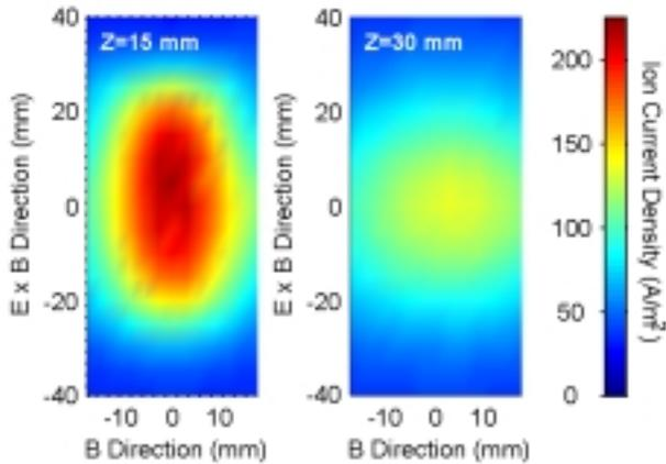
Figure 12 - Mean ion current profiles for diamond thruster.
