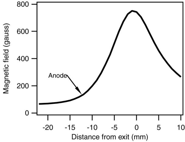
Figure 3-Magnetic field profile for the linear Hall thruster
