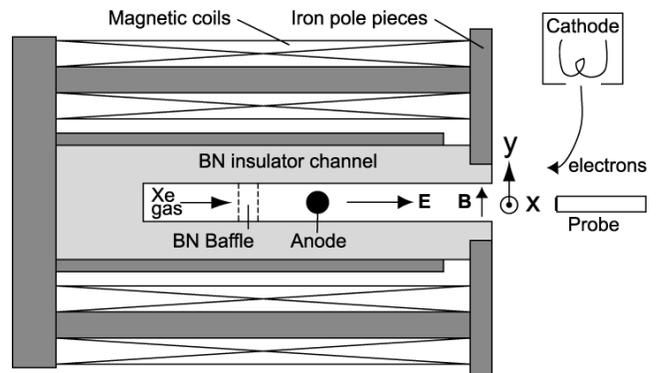
Figure 2 - Linear Hall thruster design details (BN channel)
