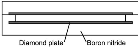
Figure 4-Schematic of diamond channel design
