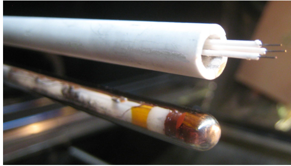
Figure 7. Triple Langmuir probe and tungsten wire tips alongside magnetic probe.
