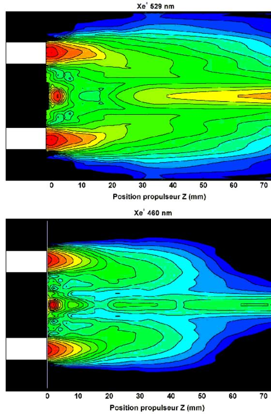
Figure 13: Xe<sup>+</sup> 529.2 nm and Xe<sup>+</sup> 460.3nm spectral line evolution in the plume.
