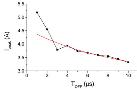
Figure 12: Evolution of the transient peak intensity with  $T_{\text{OFF}}$ .
