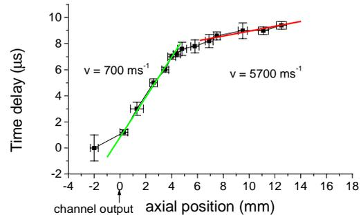
Figure 18: Evolution of the time of maximum emission along the channel.
