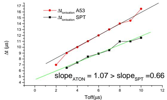
Figure 20: Variation of  $\Delta T$  for SPT and ATON structures as function of  $T_{OFF}$
