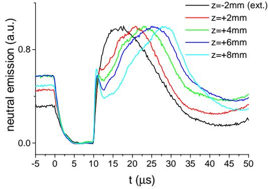
Figure 16: Normalised excitation-ionisation burst along the channel.
