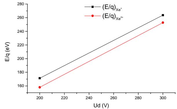
Figure 9: (energy/charge) ratio at various discharge potential
