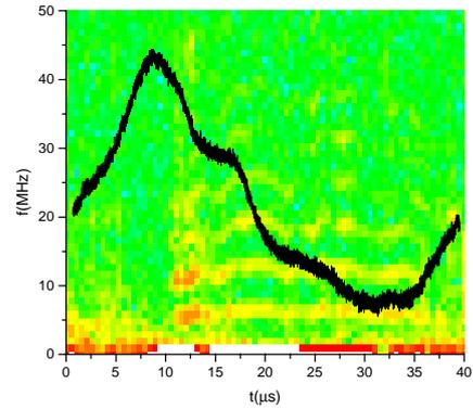
Figure 22: Discharge current and gliding Fourier transform of the inductive loop signal (single shot).
