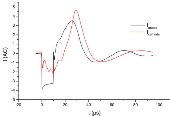
Figure 21: Cathode and anode current waveform.
