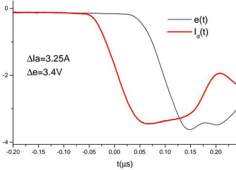
Figure 7: Discharge current and inductive loop signal when the discharge is switched off.
