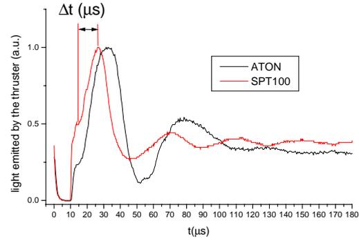
Figure 19: SPT and ATON thrusters response to a  $T_{OFF}=10\mu\text{s}$  discharge extinction.
