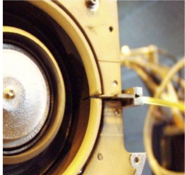
Figure 4: installation of this OFA on the thruster structure
