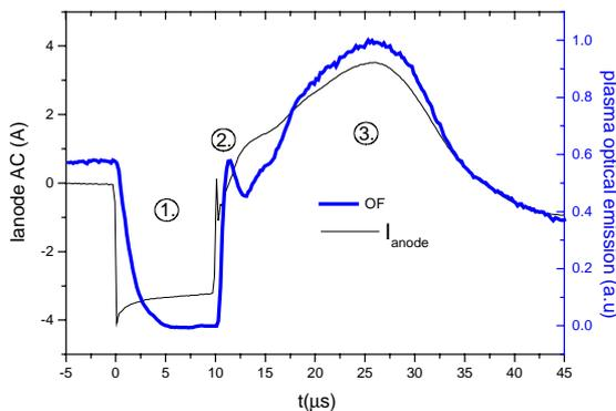
Figure 3: Discharge current and optical emission in the channel response to a current interruption.
