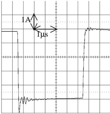
Figure 2: Discharge shutter test on a resistive charge.
