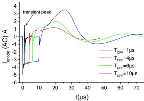
Figure 11: Evolution of the discharge current for different current interruption duration
