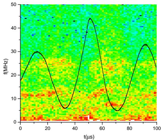
Figure 23: Discharge current and gliding Fourier transform of the inductive loop signal (average 128 triggered on  $I_d$ )
