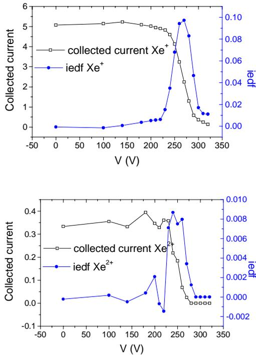
Figure 14: RPA collected current and iedf for  $\text{Xe}^+$  and  $\text{Xe}^{2+}$  ions
