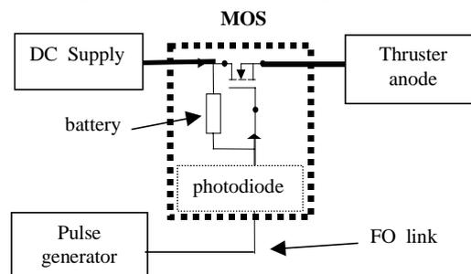
Figure 1: the discharge shutter
