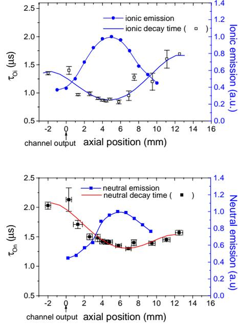
Figure 10: Evolution of the characteristic emission decay time compared to the stationary emission both for ions and neutrals.
