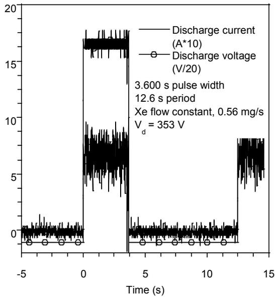
Figure 11 Discharge voltage and current versus time. 3.600 s pulse width
