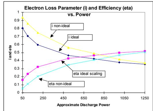
Figure 2 Electron loss parameter  $i$  and efficiency  $\eta$  are plotted versus a nominal thruster power for 2 different self similar scaling procedures. The ideal scaling is  $B$  and  $n_n$  as  $(1/L)$ , non ideal scaling which is more physically realistic is  $(1/L)^{0.75}$ . Both the ideal and nonideal scaling includes effects of wall sheath ( $k_s \lambda$ ).
