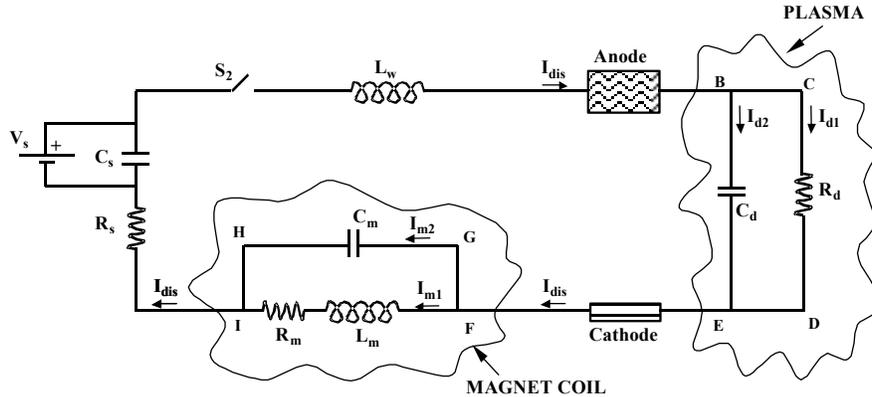
Figure 3 Electrical schematic of the capacitively driven Hall thruster
