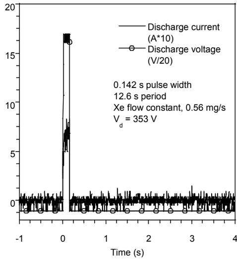
Figure 10 Discharge voltage and current versus time. 0.142 s pulse width
