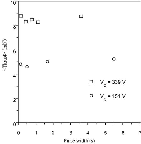
Figure 14 Average Thrust,  $\langle T \rangle = \frac{1}{P_W} \int_0^{P_W} P_W T dt$  versus pulse width
