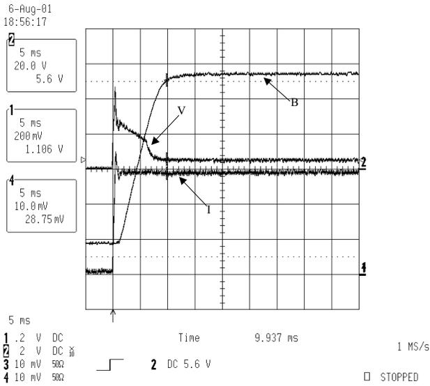
Figure 7 Measured thruster magnet coil voltage (V), current (I) and gap flux density (B) with the thruster on a bench Isp. The power supply was current limited to 1.5 A. The B increases about 6 msec after I reached steady state and required a total of 10 msec to reach a DC level. The predicted  $\tau_{md} \approx 20$  msec.
