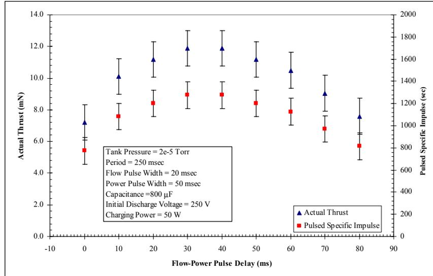
Figure 18 Thrust and Isp for a 50 msec discharge pulse. Performance peaks at a 30-40 msec delay between the flow and power trigger signals.
