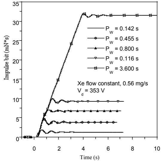
Figure 12 Time integral of balance output for different pulse width
