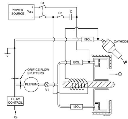
Figure 1 Schematic of the flow and power system for pulsed BHT-200
