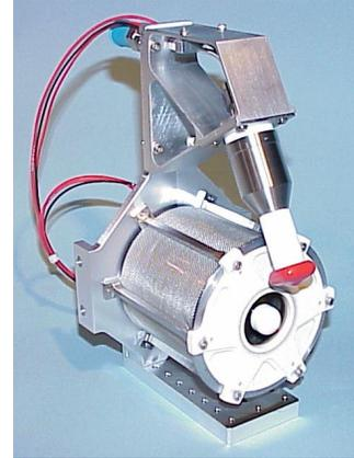
Figure 9 Photograph of the typical experimental hardware BHT-200 thruster and BHC-1500 hollow cathode. Not shown is the cathode flow isolator, essential for pulsing experiments.
