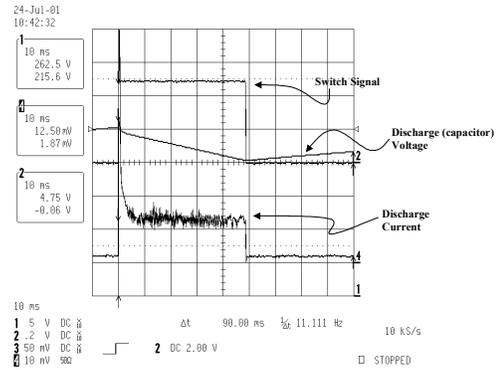
Figure 16 Typical oscilloscope traces for a 50 msec discharge pulse at the nominal steady state thruster mass flow rate.
