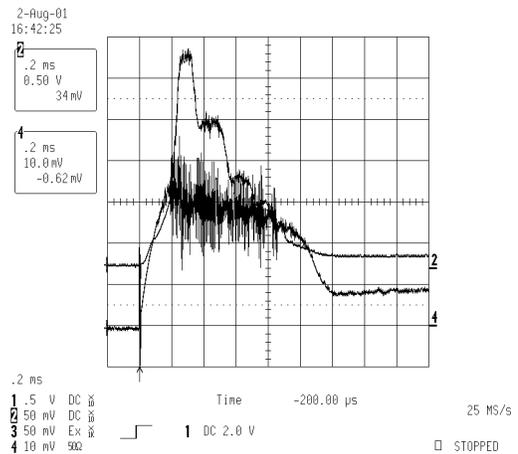
Figure 6 Measured discharge current (lower trace) using 0.8 mF capacitor and magnetic coil in series with the discharge. The upper trace is UV light output from the discharge indicating that most of the
