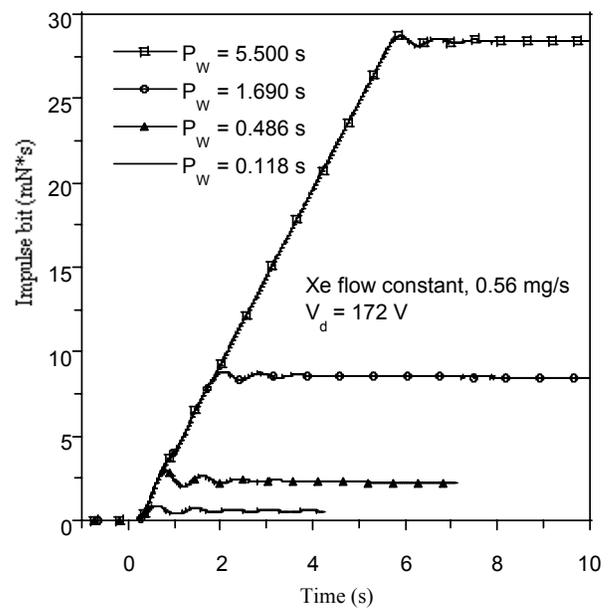
Figure 13 Time integral of balance output for different pulse widths.  $V_d = 172$  V
