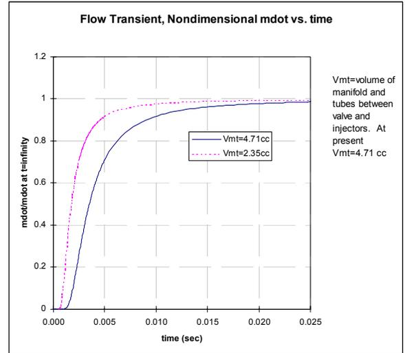
Figure 8 Predicted nondimensional thruster mass flow  $[\dot{m}_{in}(t)/\dot{m}_{in}(t = \infty)]$  is plotted versus time after the propellant valve opens. The solid line corresponds to the present set up ( $V_{mt} = 4.71$  cm<sup>3</sup>). The dashed line indicates that reducing  $V_{mt}$  by 50% reduces the filling time by about the same fraction.
