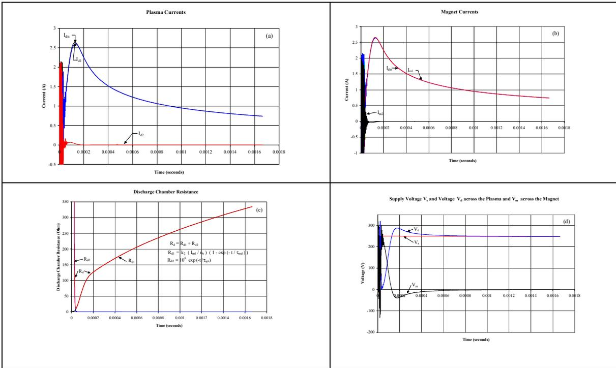
Figure 5 Start-up transients history in BHT-200 Hall thruster.  $L_w=10^{-4}H$ ,  $C_m=10^{-8}F$ ,  $C_d=1.8 \times 10^{-8}F$ ,  $\tau_{ig}=3 \times 10^{-6} \text{ sec}$ ,  $\tau_{md}=2.1 \times 10^{-2} \text{ sec}$ .
