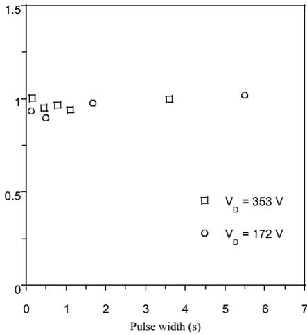
Figure 15 Ratio of average thrust,  $\langle T \rangle = \frac{1}{P_W} \int_0^{P_W} P_W T dt$  to steady state thrust versus pulse width
