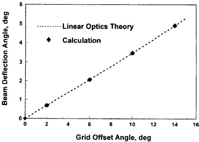
Figure 5: Beam deflection angle against grid offset angle
