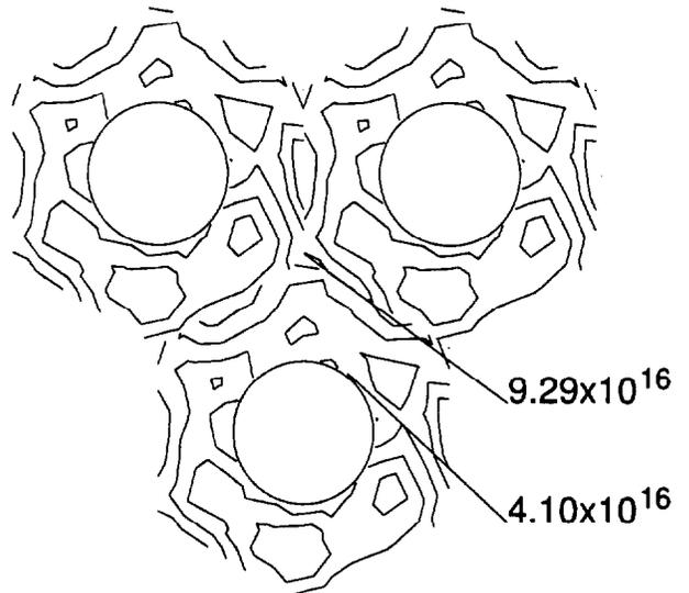
Figure 7: Erosion pattern on the downstream surface of the accelerator grid for space-based operating condition (values are number of sputtered atoms per square meters per second.)
