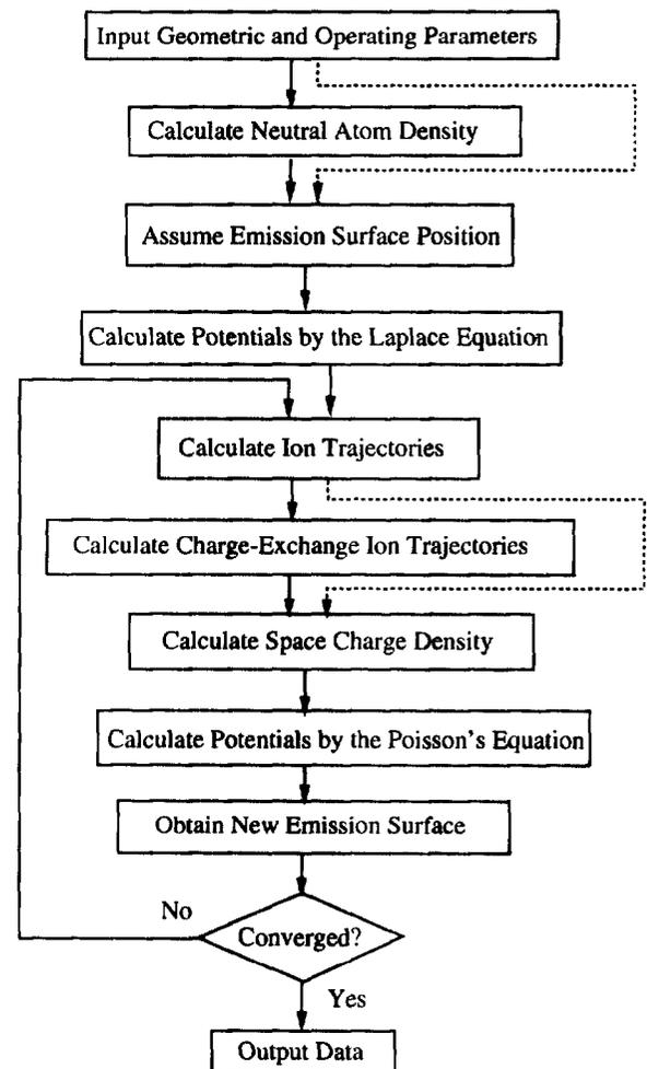
Figure 2: Block diagram of the code
