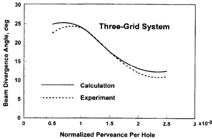
Figure 4: Beam divergence characteristics for a three-grid system
