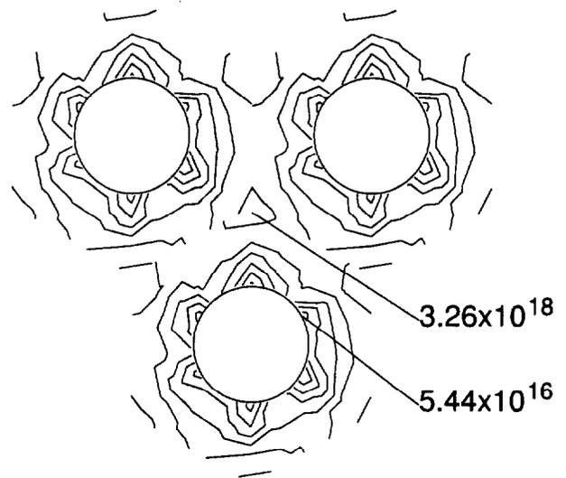
Figure 6: Erosion pattern on the downstream surface of the accelerator grid for ground-based test condition (values are number of sputtered atoms per square meters per second.)
