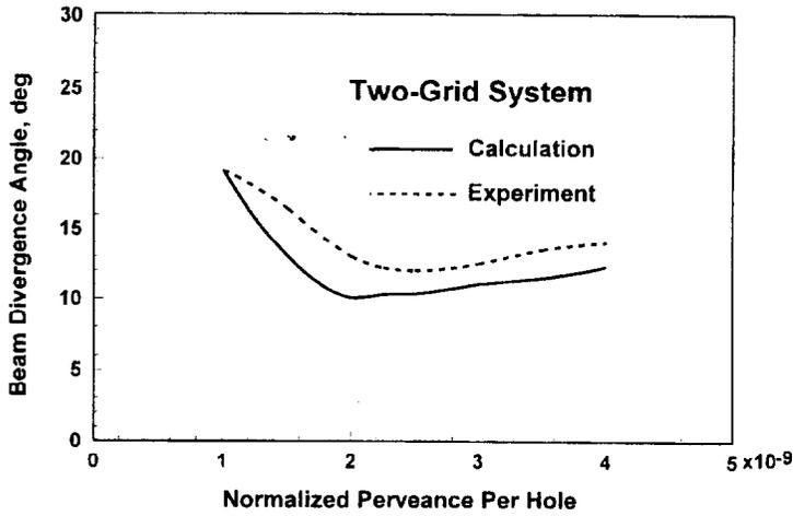
Figure 3: Beam divergence characteristics for a two-grid system
