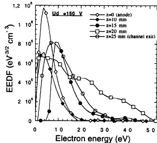
Figure 9 : EEDF inside the channel obtained with the "moving" probe at different position in the channel. The discharge voltage is 150 V and the Xenon flow rate is  $0.17 \text{ cm}^3 \text{ s}^{-1}$ .
