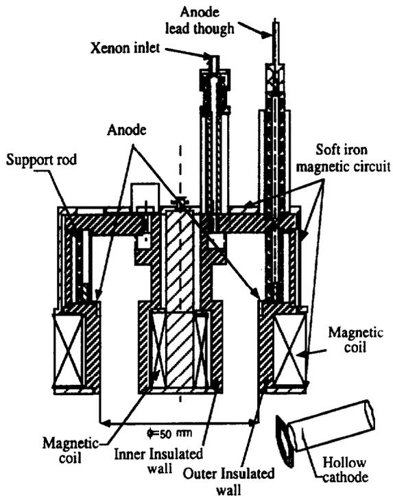
Figure 1 : The schematic representation of the Hall-type thruster SPT-50.
