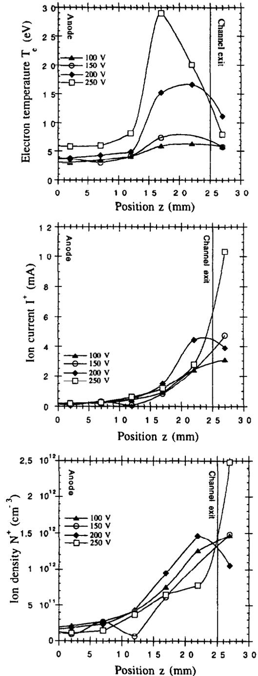
Figure 7 : Electron temperature, ion current and ion density profiles inside the SPT-50 channel obtained with the "moving" probe for different discharge voltages. Xenon flow rate is constant at  $0.20 \text{ cm}^3/\text{s}$ .
