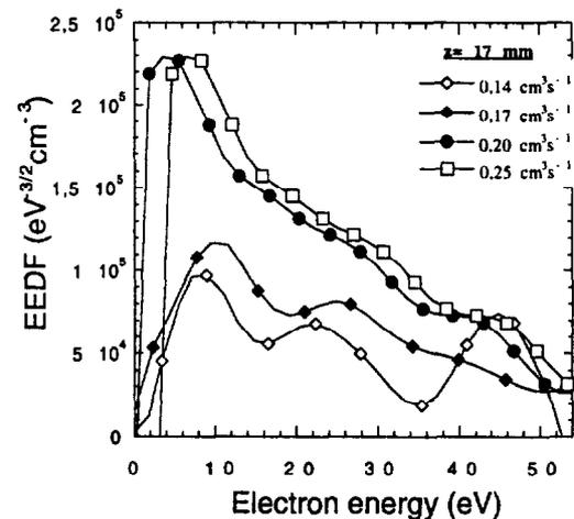
Figure 11 : Effect of the Xenon flow rate on EEDF inside the channel for  $z=0$  ("pre-ionization" region) and  $z=17 \text{ mm}$  ("ionization" region).
