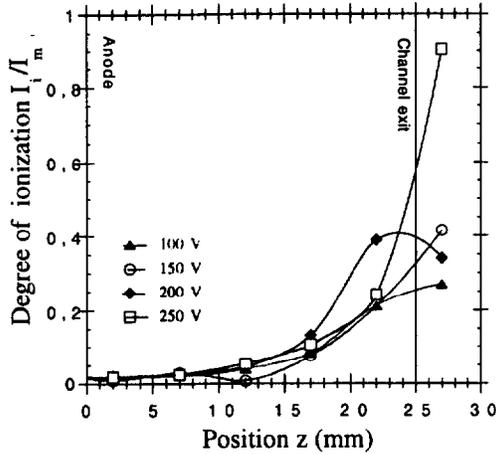
Figure 8 : Profiles of degree of ionization along the channel for different discharge voltages.
