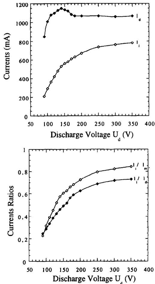
Figure 4 : Effect of discharge voltage on the discharge current,  $I_d$ , the ion current  $I_i$ , the electric efficiency  $I_i/I_d$  and the degree of ionisation  $I_i/I_m$ . The xenon gas flow is  $1.07 \text{ mgs}^{-1}$  in the anode and  $0.34 \text{ mgs}^{-1}$  in the cathode. The internal coil current is 2.1 A, the external coil current is 4.2 A.
