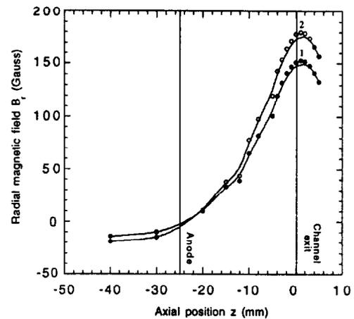
Figure 3 : Distribution of the radial magnetic field inside the channel.  $I_{m\text{int}}, I_{m\text{ext}}$  (A) : 1) 1,4 - 2,8 A. 2) 2 - 4 A
