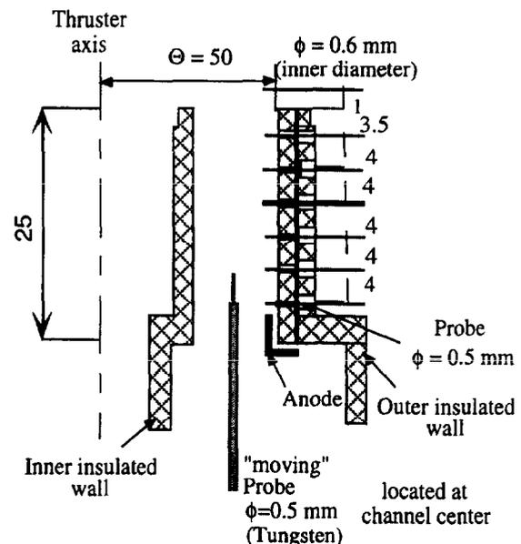
Figure 5 : Experimental setting of electrostatic probes inside the SPT-50 thruster.
