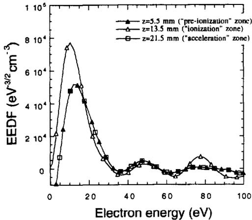
Figure 12 : axial profiles of EEDF close to the walls for three locations inside the channel.
