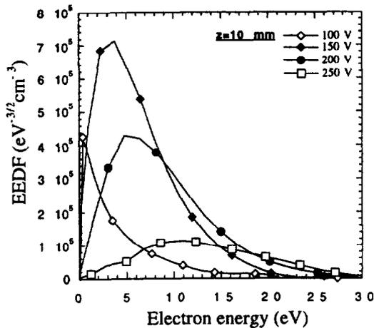
Figure 10 : Effect of the discharge voltage on EEDF inside the channel for  $z=10 \text{ mm}$  ("pre-ionization" region).
