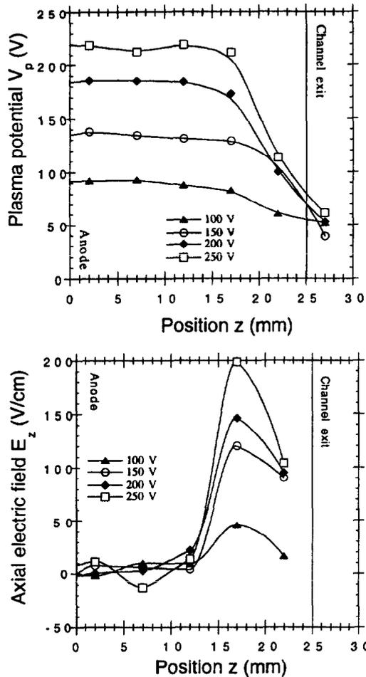
Figure 6 : Plasma potential and electric field profiles inside the SPT-50 channel obtained with the "moving" probe for different discharge voltages. Xenon flow rate is constant at  $0.20 \text{ cm}^3/\text{s}$ .
